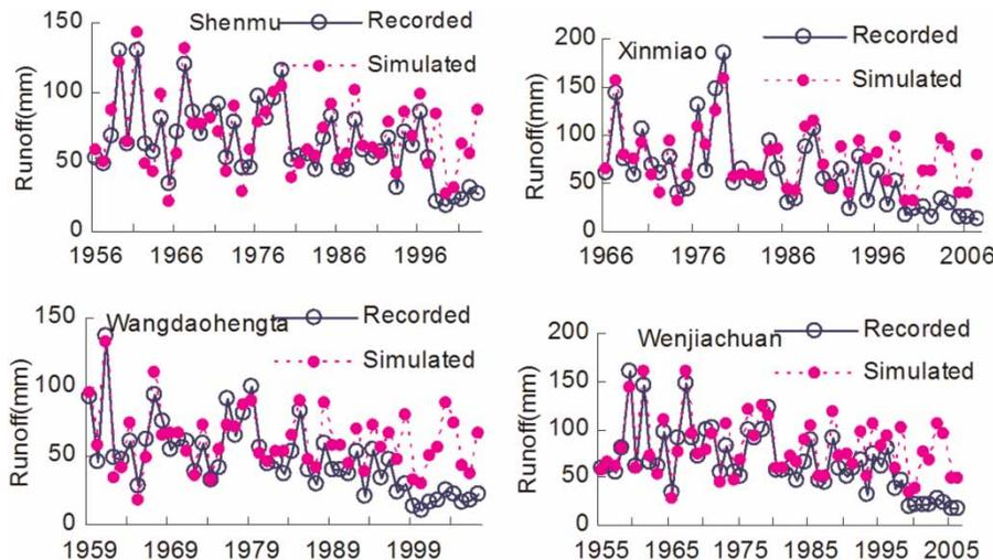
Figure 6 | Simulated and recorded annual runoff at hydrometric stations in the Kuye River catchment.
