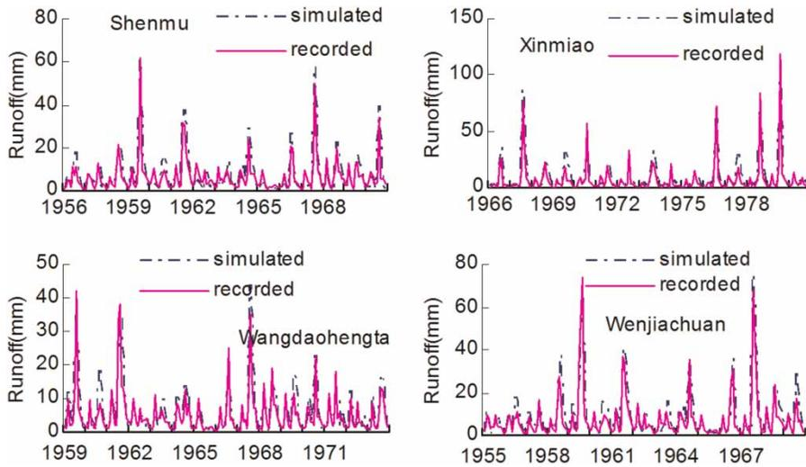
Figure 5 | Monthly recorded and simulated runoff at hydrometric stations in the Kuye River catchment.
