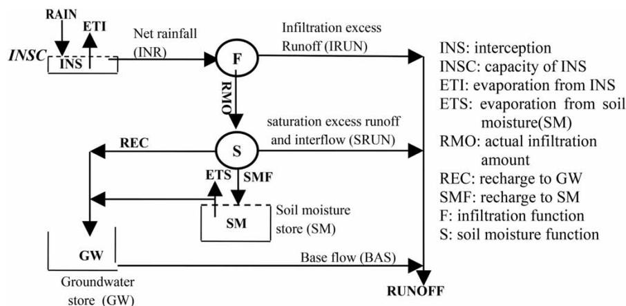
Figure 2 | Schematic diagram of the SimHyd rainfall runoff model.
