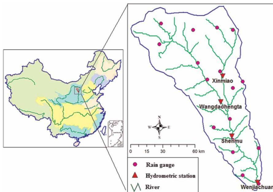
Figure 1 | River system and location of rain gauges and hydrometric stations in the Kuye River catchment.
