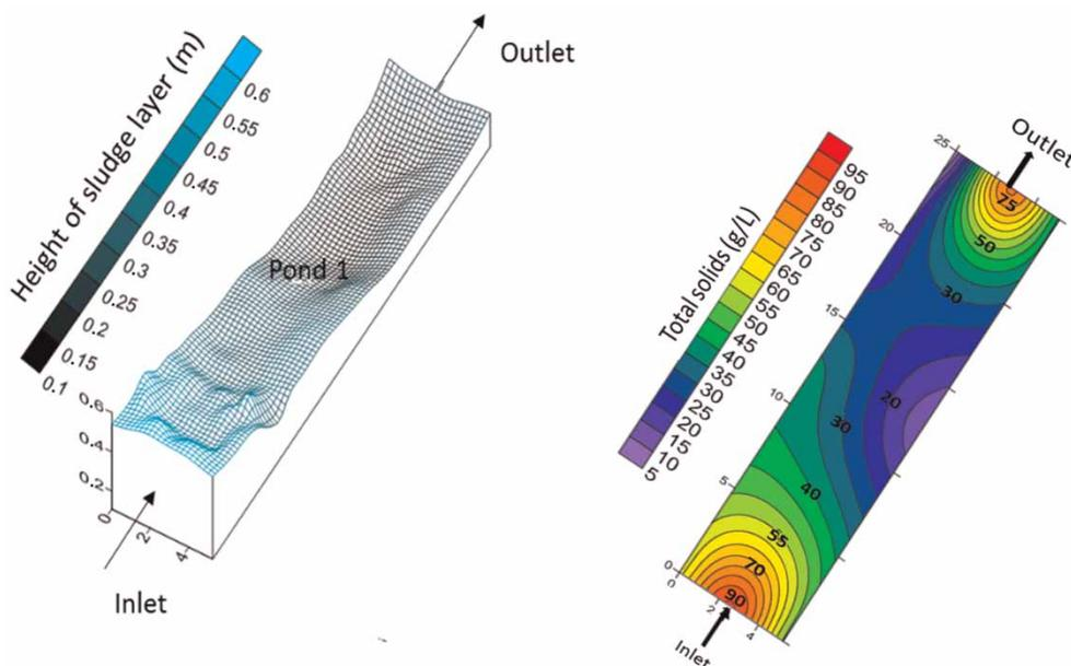
Figure 2 | Distribution of the height of the sludge layer (left) and TS concentration (dry matter) in the sludge (right) in Pond 1, after 11 years of operation.
