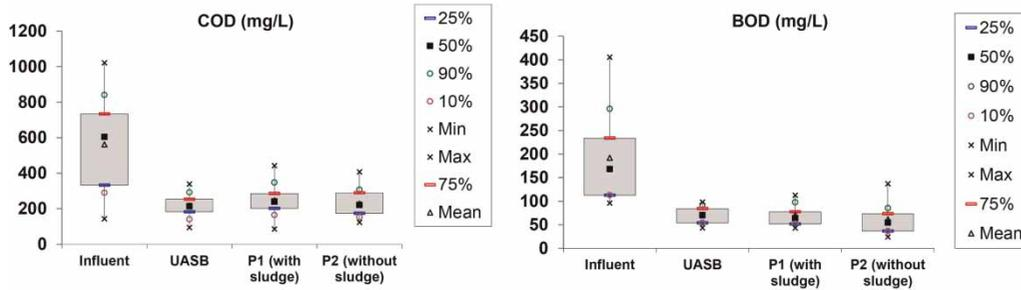
Figure 4 | Box-plot of total organic matter (COD and BOD concentrations) in the raw sewage and effluents from the UASB reactor and both ponds.
