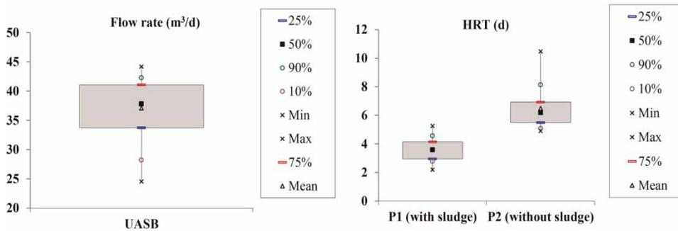
**Figure 3** | Box-plot of the flow rate of the effluent from the UASB reactor and the theoretical HRT in the ponds with (P1) and without (P2) sludge.
