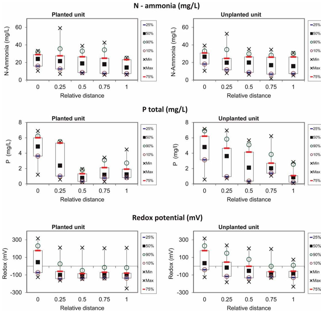
**Figure 3** | Box-plots of the longitudinal profile of N-ammonia (top), phosphorus (middle) and redox potential (bottom) along the length of both wetland units.
