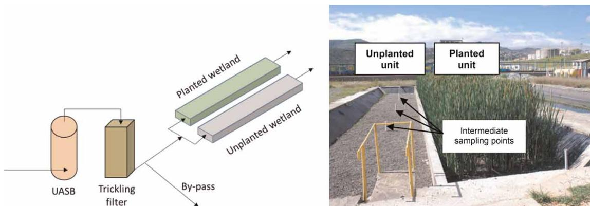
**Figure 1** | Flowsheet of the treatment system (left) and view of the two wetland units (right).
