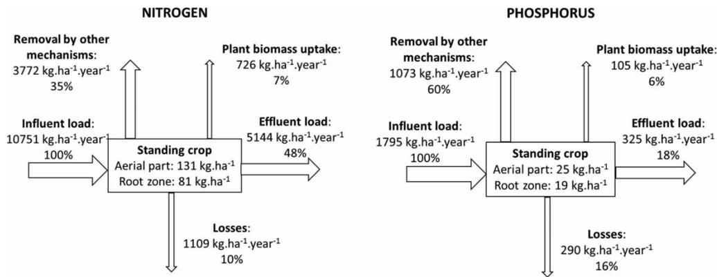
Figure 4 | Mass balance of nitrogen and phosphorus in the planted wetland.
