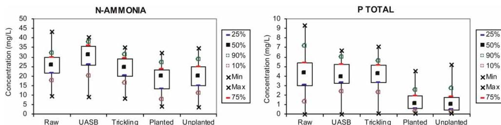
**Figure 2** | Box-plots of ammonia and total P concentrations in the units along the treatment system.
