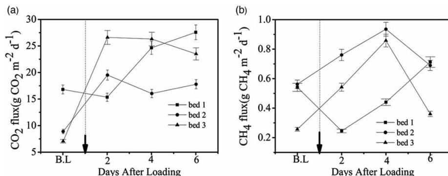
**Figure 4** Fluxes of CO<sub>2</sub> (a) and CH<sub>4</sub> (b) before loading (B.L.) of sludge and 2, 4 and 6 days after loading in the STRBs. The black arrows indicate the time of sludge loading. B.L. represents pooled data from three sampling events before loading.
