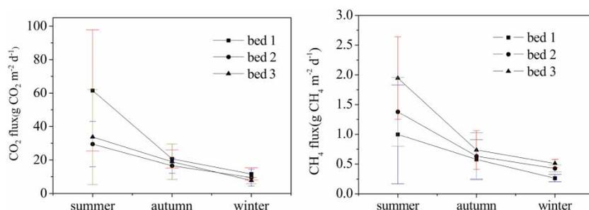
Figure 3 | Rates of CO<sub>2</sub> (a) and CH<sub>4</sub> (b) emissions through the bed surfaces during the 2013 vegetation season.
