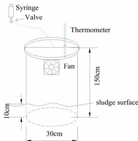
**Figure 2** | Diagram of a closed gas sampling chamber (Livingston & Hutchinson 1995).
