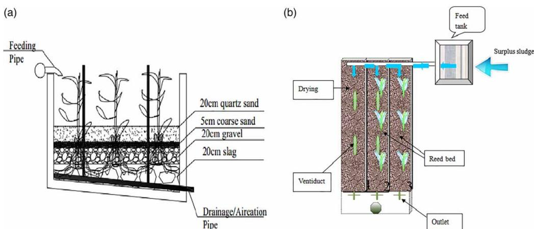
**Figure 1** | (a) Schematic diagram of an STRB planted with reeds. (b) Schematic drawing of the whole STRB system: the beds are consecutively numbered from left to right, 1, 2 and 3. Bed 1 was plant-free. Beds 2 and 3 were planted with common reed. Beds 1 and 2 were set with aeration pipes, while Bed 3 had no aeration pipe.
