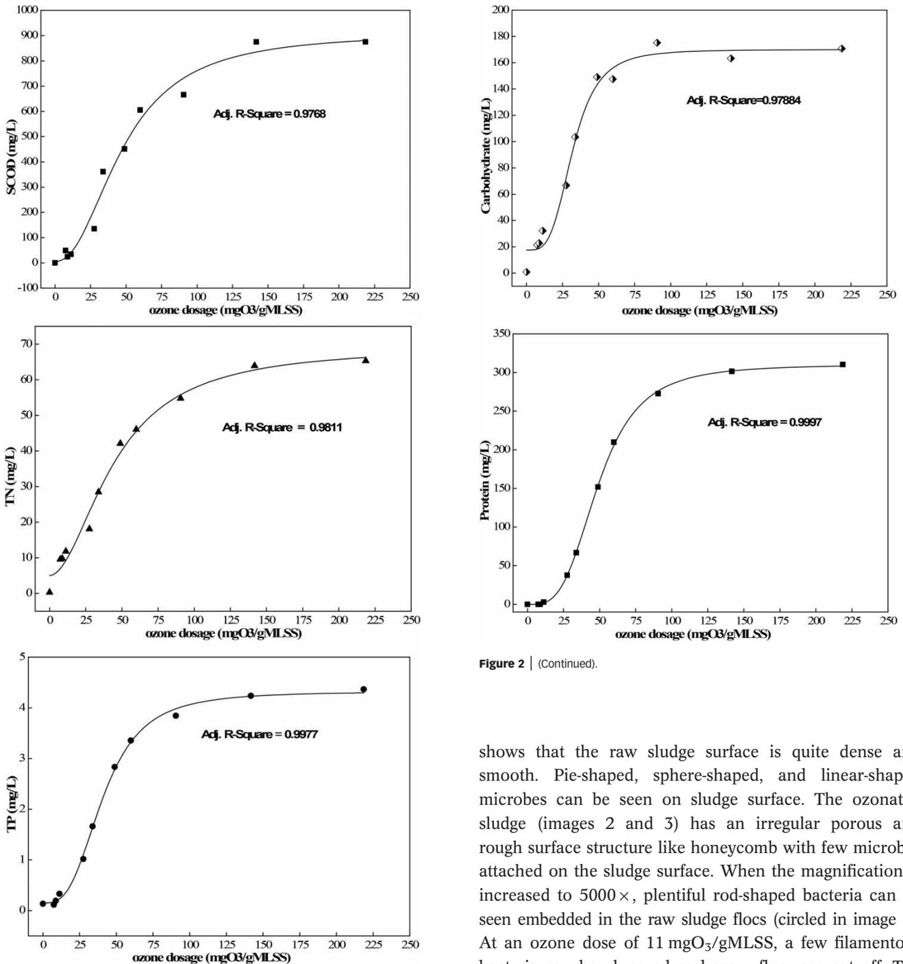
**Figure 2** | Solubilization of SCOD, TN, TP, carbohydrate and protein during sludge ozonation.
