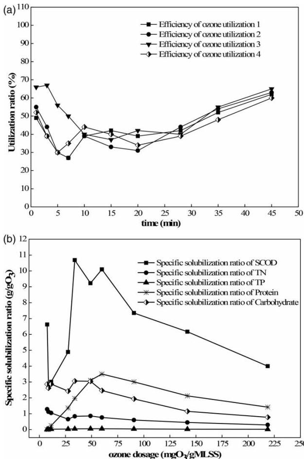
Figure 4 | (a) Efficiency of ozone utilization in four parallel experiments. (b) Specific solubilization ratio of SCOD, TN, TP, protein and carbohydrate.
