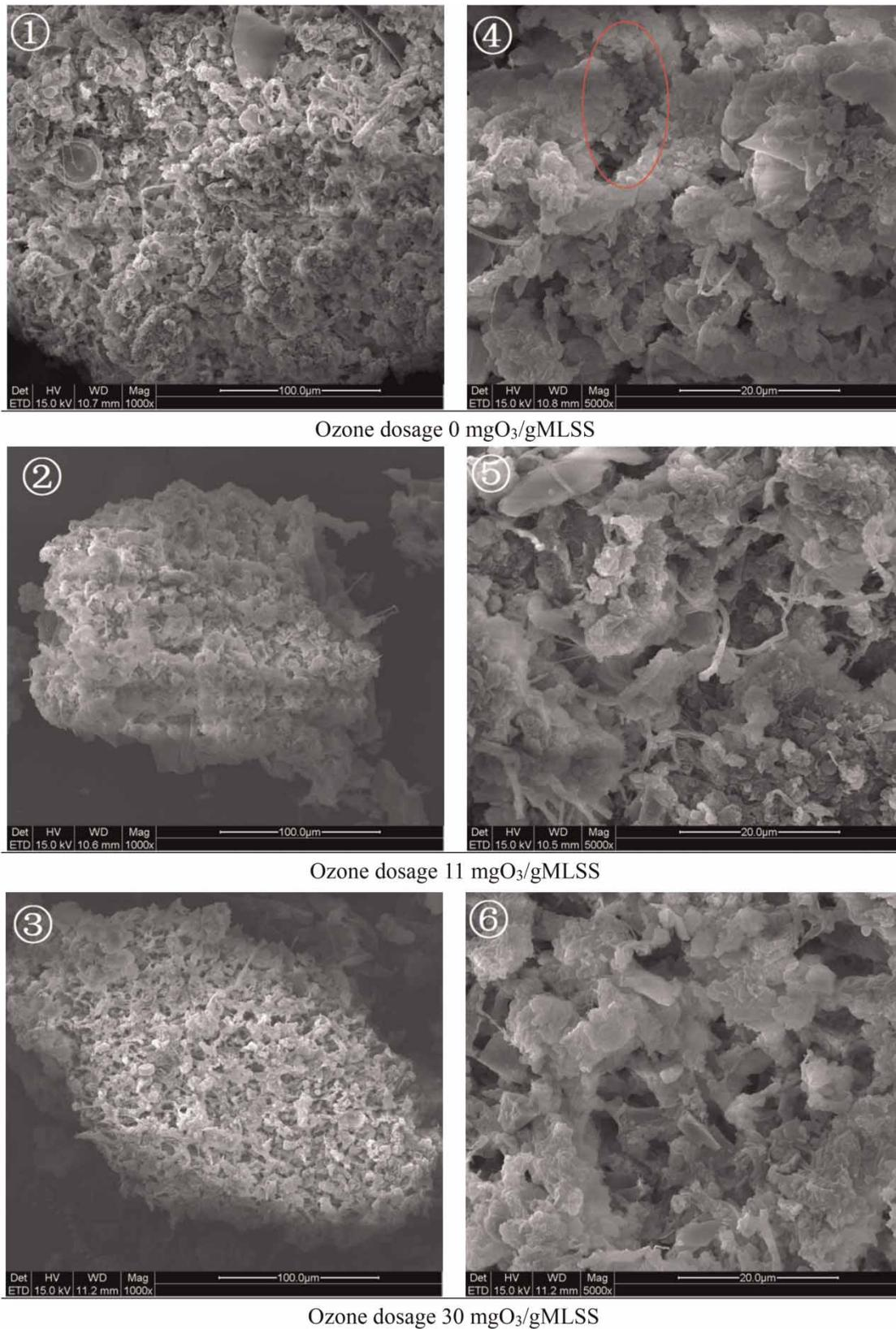
Figure 3 | SEM images of sludge at different ozone dose (right  $\times 1000$ ; left  $\times 5000$ ).
