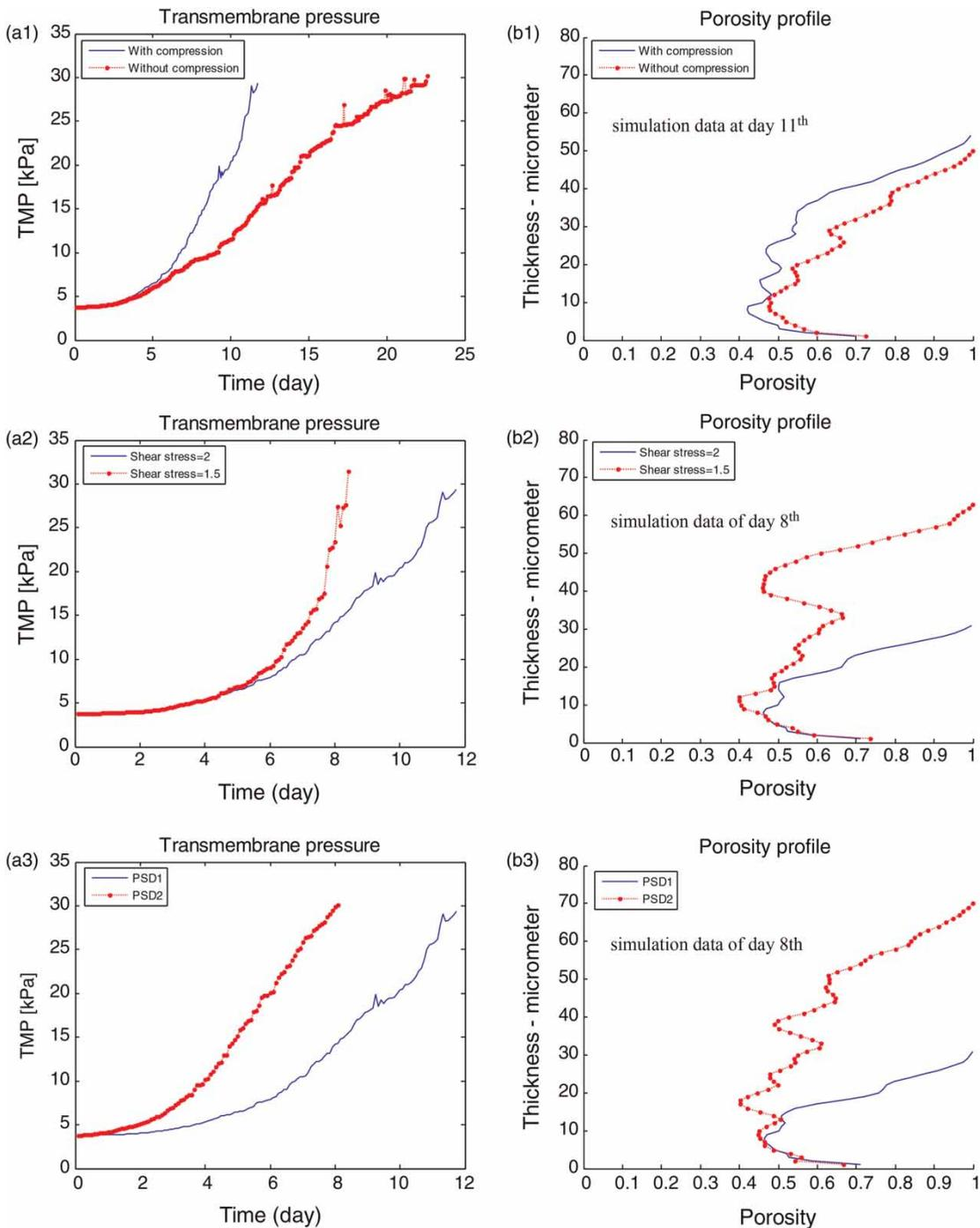
**Figure 4** | Influence of compression, shear stress and PSD on (a) the TMP profile (b) the porosity profile at the flux of 27 L/m<sup>2</sup>·h.
