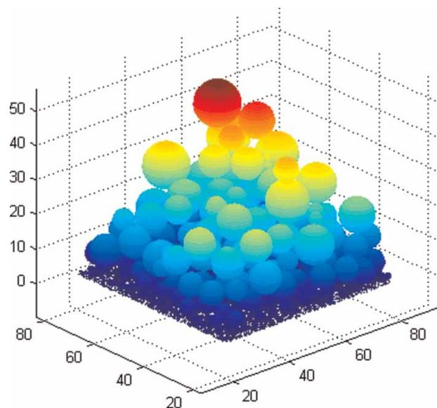
Figure 2 | 3D cake layer with multi-size particles after filtration.
