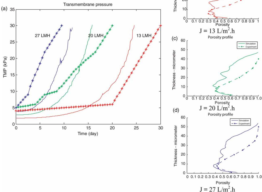
Figure 3 | Comparisons of the TMP and porosity profile between experimental and simulated data (\*: experimental data, —: simulated data).
