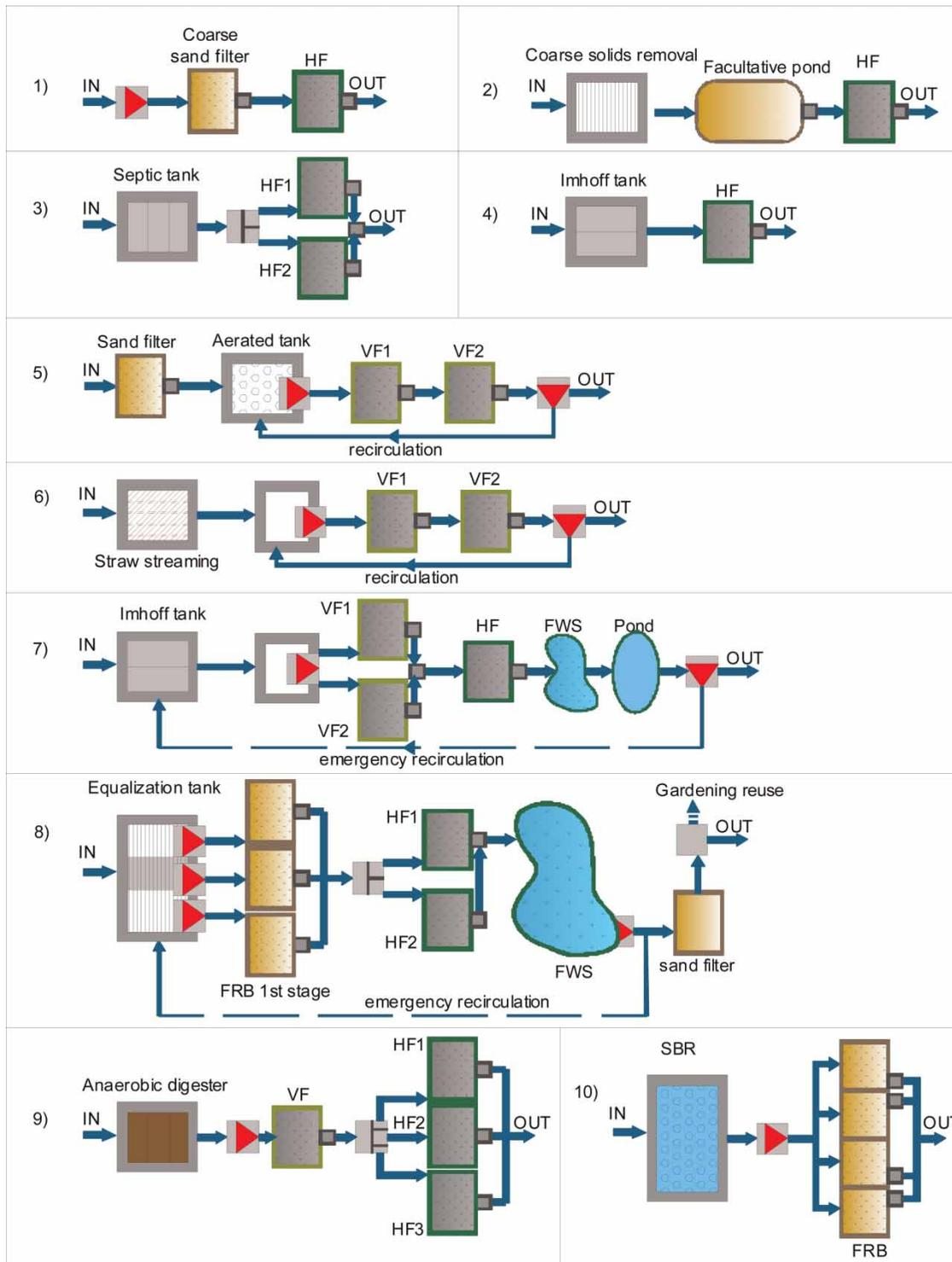
**Figure 1** | Adopted treatment approaches for wineries CWs (the numbers in each box correspond to the IDs in Table 2).
