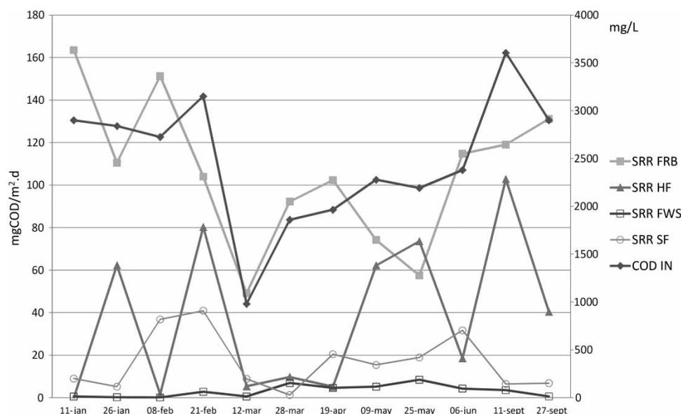
Figure 3 | SRR for the different stages of the Cecchi winery MTW versus COD inlet concentration (Masi et al. 2014).
