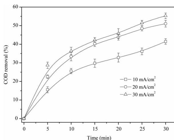
**Figure 1** | Effect of current density on COD removal of effluent at the surface of  $\beta$ - $PbO_2$  anode. Conditions: pH 5.0 and conductivity 8.0 mS/cm.
