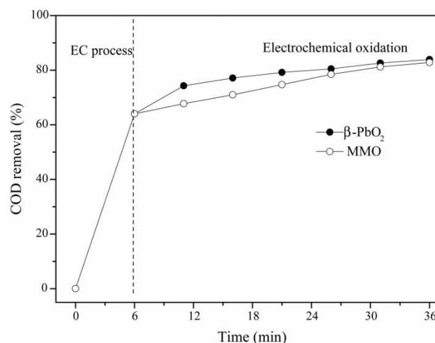
**Figure 3** | Evolution of COD removal during the combined process. Conditions: EC process: current density 40 mA/cm<sup>2</sup>, reaction time 6 minutes, and pH 6.8. Electrochemical oxidation: reaction time 30 minutes, current density 20 mA/cm<sup>2</sup> ( $\beta$ -PbO<sub>2</sub>) and 30 mA/cm<sup>2</sup> (MMO), and pH 5.0 ( $\beta$ -PbO<sub>2</sub>) and 6.7 (MMO).
