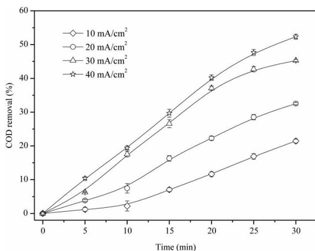
**Figure 2** | Effect of current density on COD removal of effluent at the surface of MMO anode. Conditions: pH 6.7 and conductivity 8.0 mS/cm.
