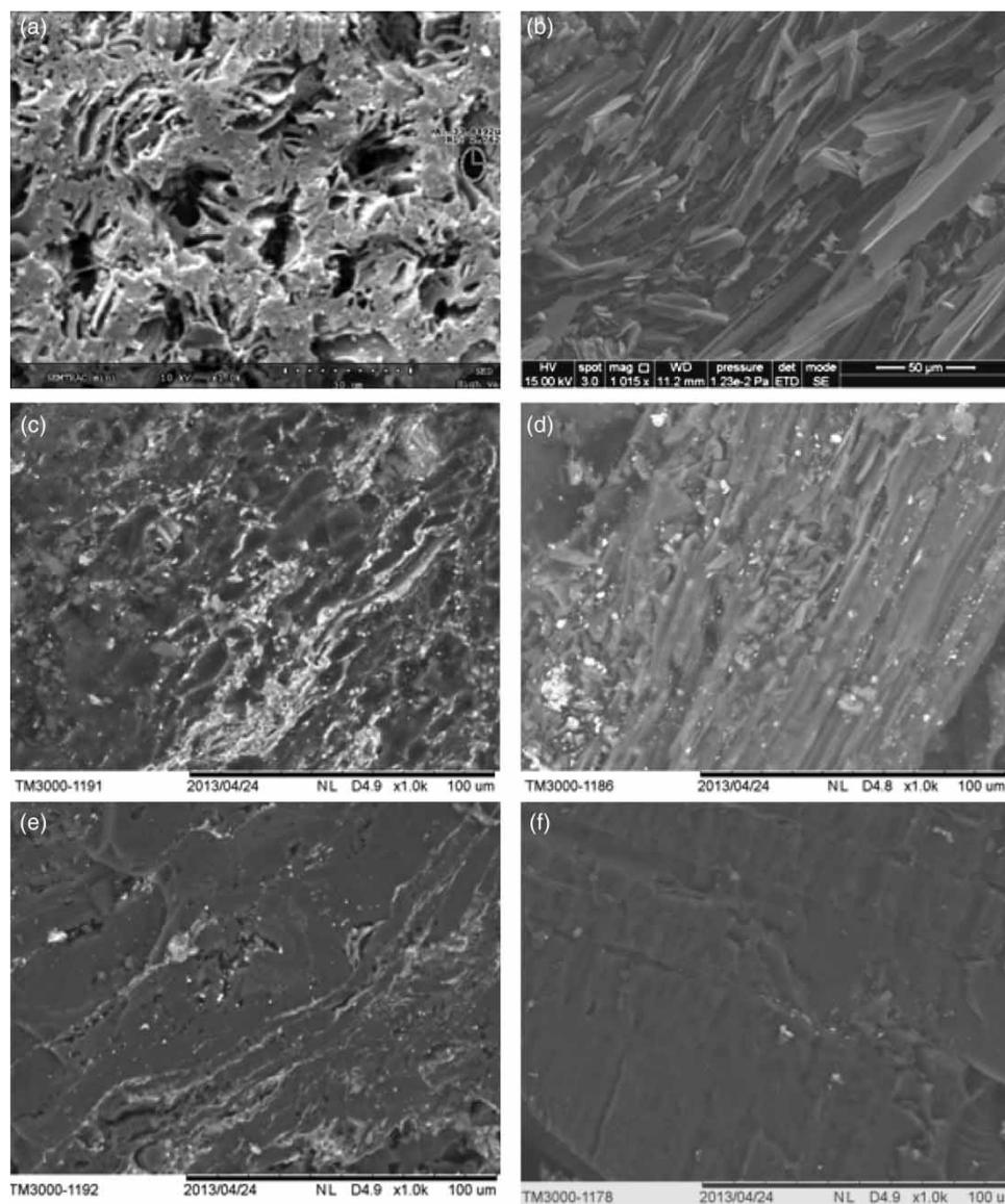
Figure 1 | SEM images of the prepared ACs: (a) AC-I; (b) AC-II; (c) AC-III; (d) AC-IV; (e) AC-V; (f) AC-VI.
