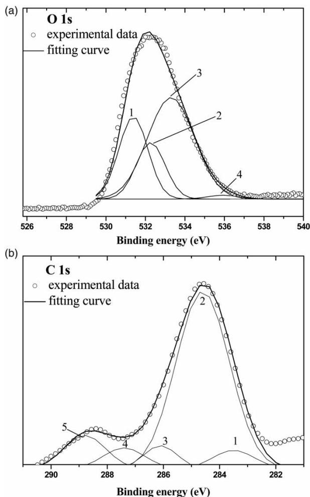
**Figure 3** | (a) XP O1s core level spectra of the AC-I materials: (1) C=O; (2) C–OH, C–O–C; (3) C–O–C=O; (4) chemisorbed water, (b) XP C1s core level spectra of the carbon materials: (1) carbidic; (2) graphitic; (3) C–OH, C–O–C; (4) C=O; (5) C–O–C–O.
