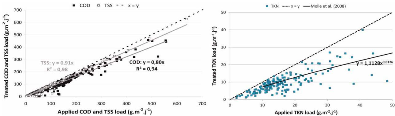
**Figure 4** | Treated COD, TSS (left) and TKN (right) loads according to the COD, TSS and TKN loads applied to the first stage of VFCW system.  $N = 190$  for COD and TSS loads;  $N = 174$  for TKN loads.
