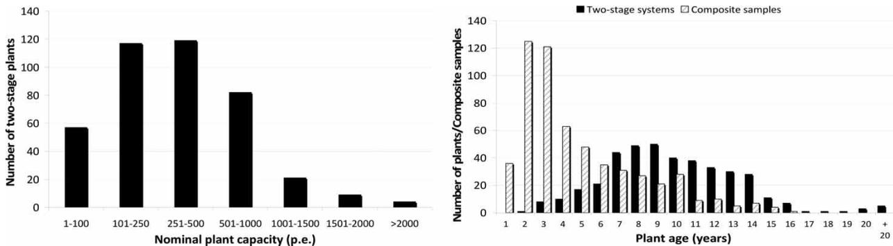
**Figure 1** | Distribution of the number of two-stage systems according to nominal plant capacity (left). Distribution of the number of composite samples and the number of two-stage systems according to plant age (right).
