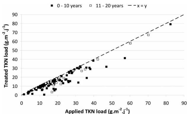
**Figure 5** | Treated TKN loads according to the TKN loads applied to the first stage of old VFCW plants (aged from 13 to 20 years) according to the age of the plants when the composite samples were made.  $N = 131$ .
