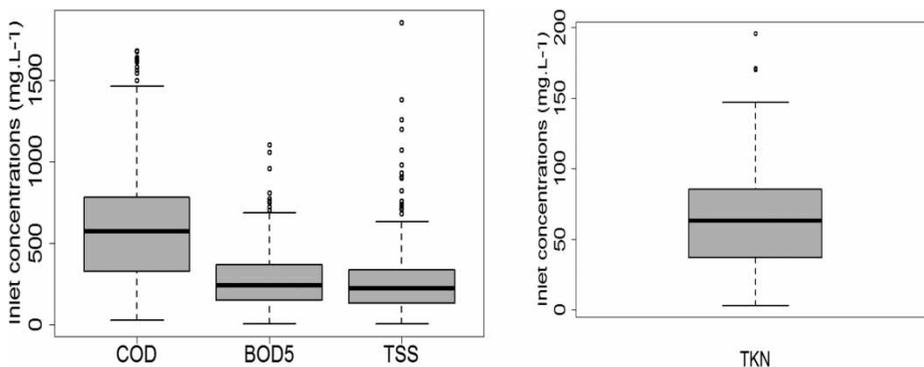
**Figure 2** | Raw wastewater concentrations (COD, BOD<sub>5</sub> and TSS on the left; TKN on the right) applied to the two-stage VFCW system.  $N = 394$ ,  $N = 386$ ,  $N = 397$  and  $N = 325$  for COD, BOD<sub>5</sub>, TSS and TKN, respectively.  $N$ : the number of values.
