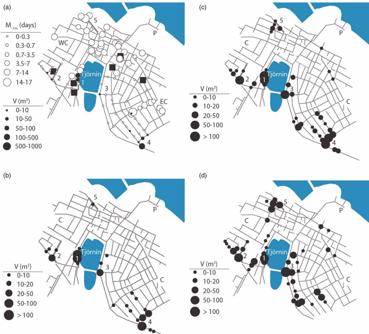
**Figure 3** | Locations of flooded manholes in MIKE URBAN scenarios. (a) ARS, (b) CDS, (c) CDS-R and (d) CDS-RD. Water-related property damage locations are indicated as squares.
