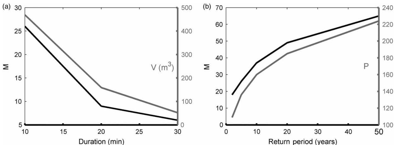
Figure 4 | Flooding indicators for CDS with rainfall peaks of varying (a) duration and (b) return period.
