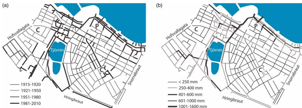
Figure 1 | The modelled combined sewer network located in downtown Reykjavik. (a) Pipe age. (b) Pipe diameter.
