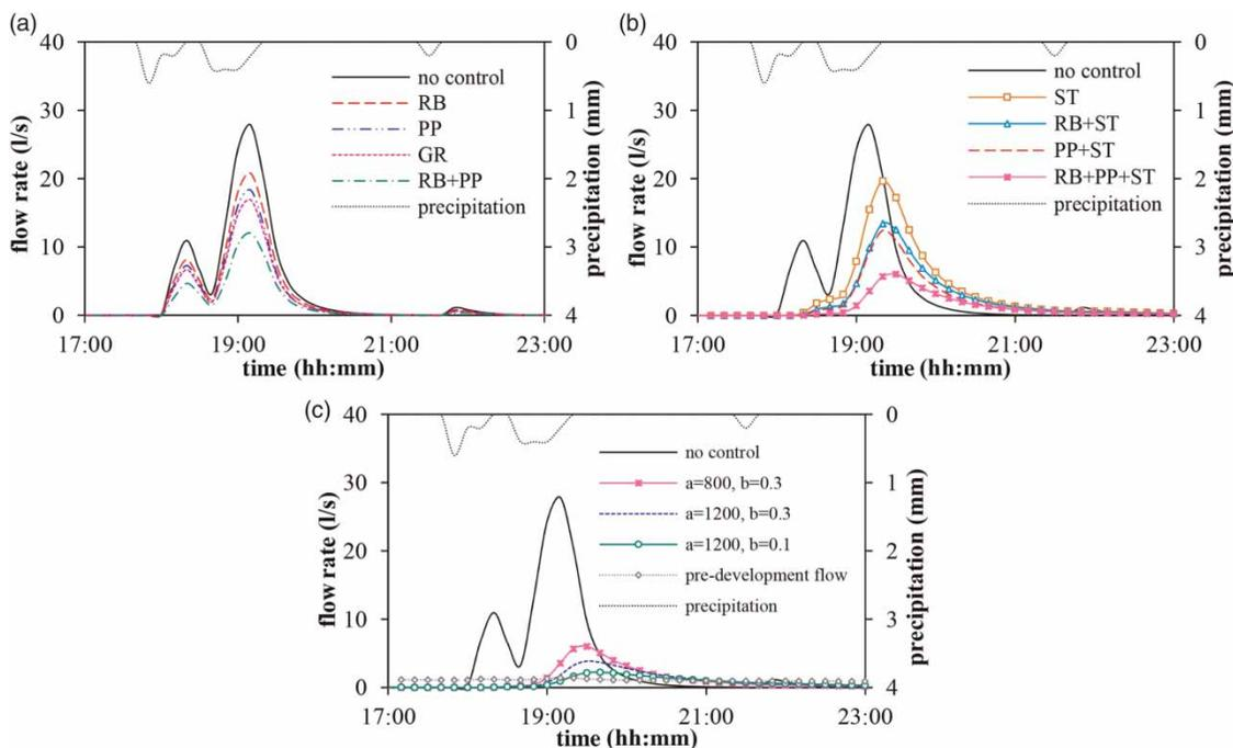
**Figure 2** | The simulated hydrographs without and with different LID controls for E1, and the observed pre-development flow.
