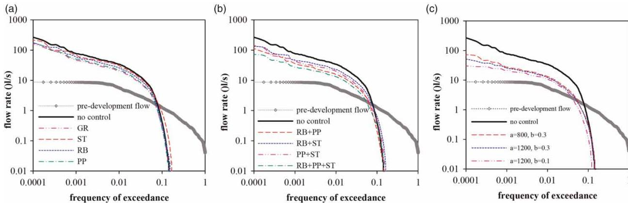
**Figure 4** | Simulated flow-frequency curves for the fully developed catchment without LID and with LID controls, and the observed pre-development flow-frequency curve for the continuous scenario E5; the intersection between the curve and the y-axis shows the maximum peak flow during the simulation period, and the intersection with the x-axis shows the fraction of time during which a flow is detected at the outlet.
