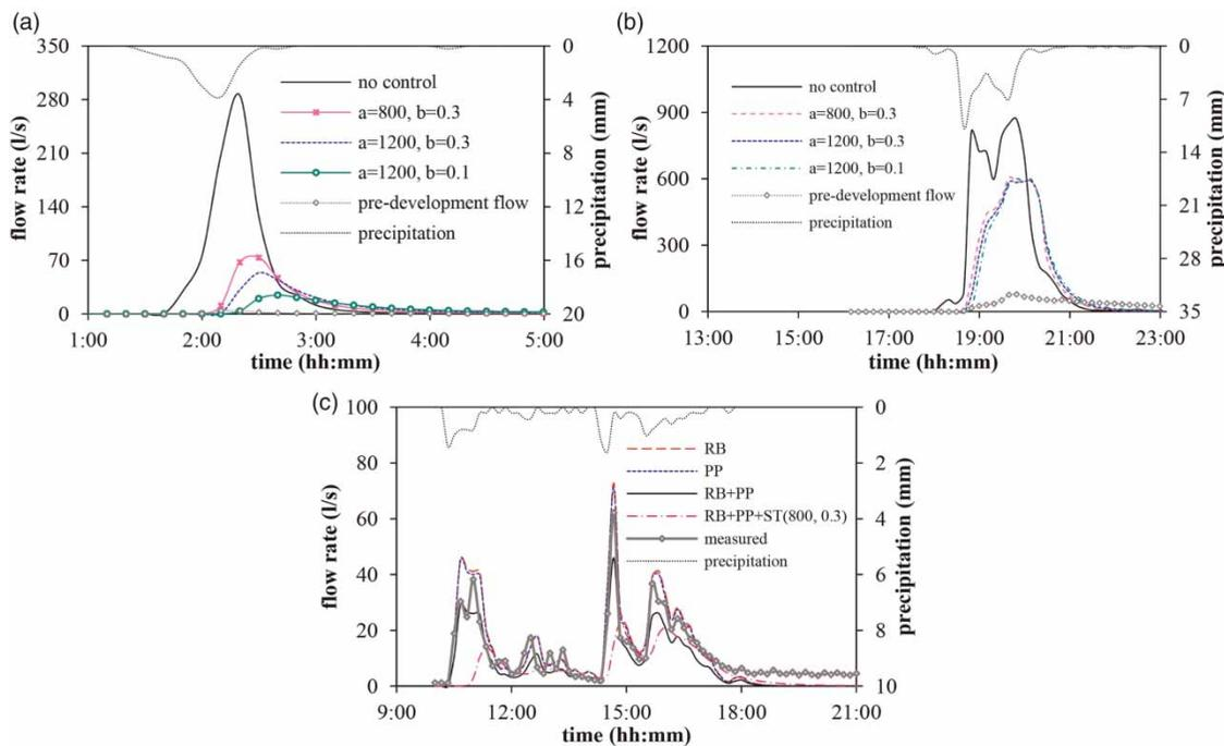
**Figure 3** | The simulated LID hydrographs for the fully developed catchment and the observed pre-development flow for (a) E2 and (b) E3; (c) the simulated LID hydrographs and the measured hydrographs for partially developed catchment conditions for E4.
