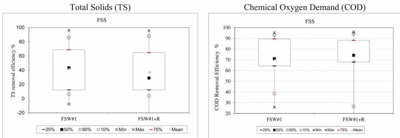
**Figure 3** | Box-plot of TS and COD removal efficiencies during Phase 2 in the full-scale unit (FSS), without (FSW1) and with (FSW1 + R) percolate recirculation.
