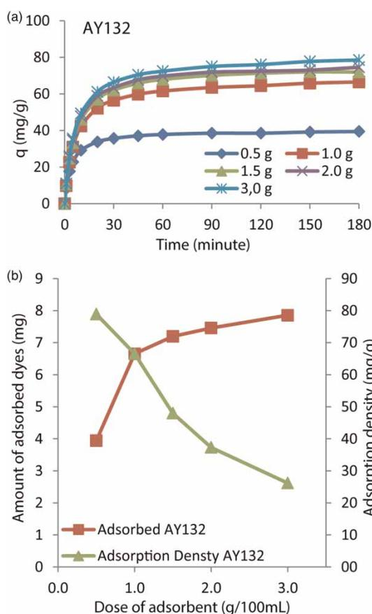
**Figure 4** | The effects of sorbent dosage on AY132 adsorption (a) and adsorption density (b) ( $C_0 = 100 \text{ mg L}^{-1}$ ,  $298 \text{ K}$ , contact time: 180 minutes,  $\text{pH} = 2$ , particle size:  $150\text{--}500 \mu\text{m}$ , 600 rpm, 100 mL).
