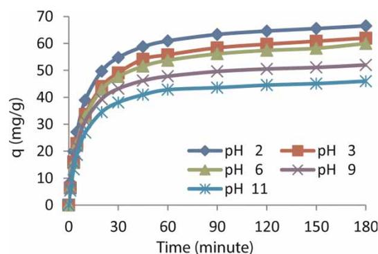
**Figure 2** | The effects of pH on AY132 adsorption ( $C_0 = 100 \text{ mg L}^{-1}$ , 298 °K, dose: 1 g/100 mL, stirring rate: 600 rpm, particle size: 150–500  $\mu\text{m}$ ).
