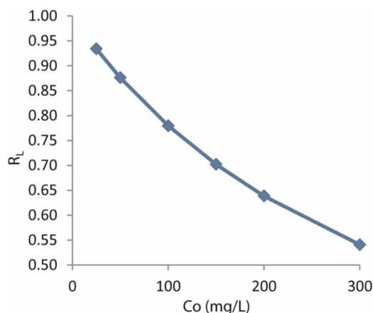
Figure 7 | Plots of separation factor versus initial dye concentrations.
