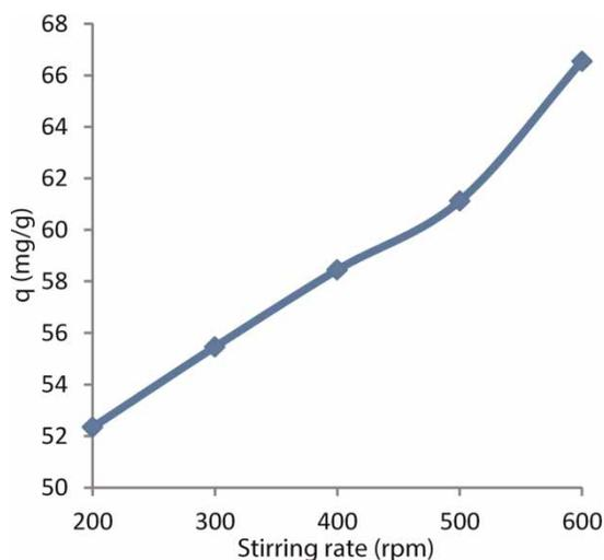
**Figure 3** | The effects of stirring rate on AY132 adsorption ( $C_0 = 100 \text{ mg L}^{-1}$ ,  $298 \text{ K}$ , dose:  $1 \text{ g}/100 \text{ mL}$ , contact time: 180 minutes,  $\text{pH} = 2$ , particle size:  $150\text{--}500 \mu\text{m}$ ).
