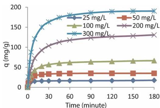
**Figure 5** | The effects of initial dye concentration on AY132 dye sorption (298 °K, pH = 2, particle size: 150–500  $\mu\text{m}$ , 600 rpm, 1 g of sorbent).
