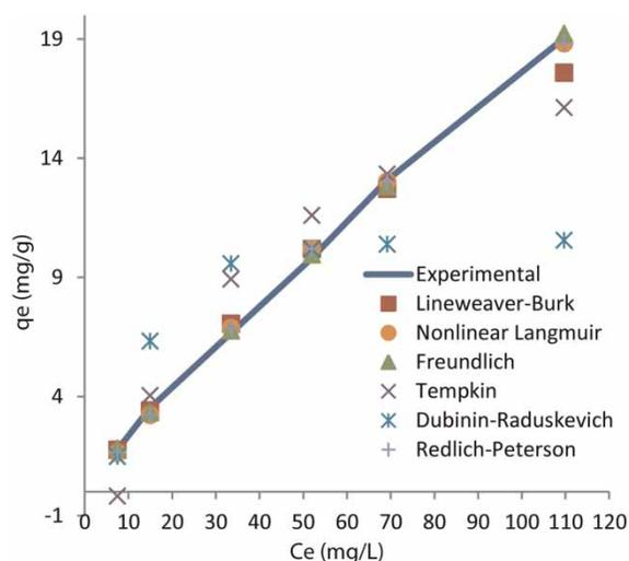
Figure 8 | Equilibrium curves for adsorption of AY132 onto red pine sawdust ( $C_0 = 25\text{--}300$  mg L $^{-1}$ , 298 °K, 180 minutes., pH = 2, 150–500  $\mu$ m particle size, 600 rpm, 100 mL, 1 g adsorbent).
