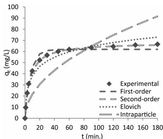
**Figure 6** | The measured and non-linear modeled time profiles for biosorption of AY132 dye at 100 mg/L initial dye concentration onto red pine sawdust at a temperature of 298 °K.
