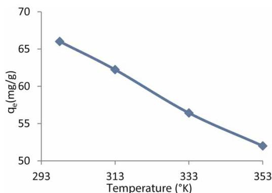
Figure 9 | Effect of temperature on AY132 dye adsorption. ( $C_0 = 100$  mg L $^{-1}$ , 180 minutes, pH = 2, 150–500  $\mu$ m particle size, 600 rpm, 100 mL, 1 g adsorbent).
