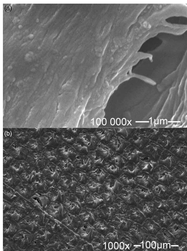
Figure 12 | FESEM micrograph of AY132 adsorbed (a) and natural (b) red pine sawdust particles (10 kV).
