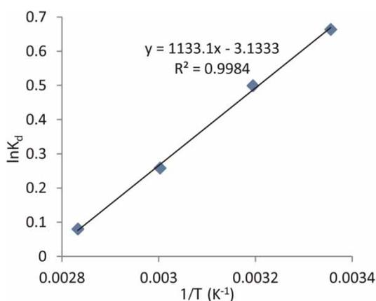
**Figure 10** | Van 't Hoff plot of  $\ln K_d$  versus  $1/T$  for the estimation of thermodynamic parameters.
