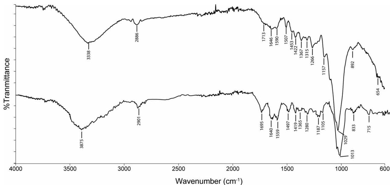
Figure 11 | FTIR spectra of sawdust and AY132 adsorbed sawdust.
