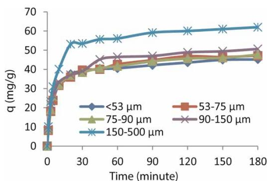
**Figure 1** | The effects of biosorbent particle size on AY132 adsorption (pH: 6.3,  $C_0 = 100 \text{ mg L}^{-1}$ , temperature: 298 °K, dose: 1 g/100 mL, stirring rate: 600 rpm).
