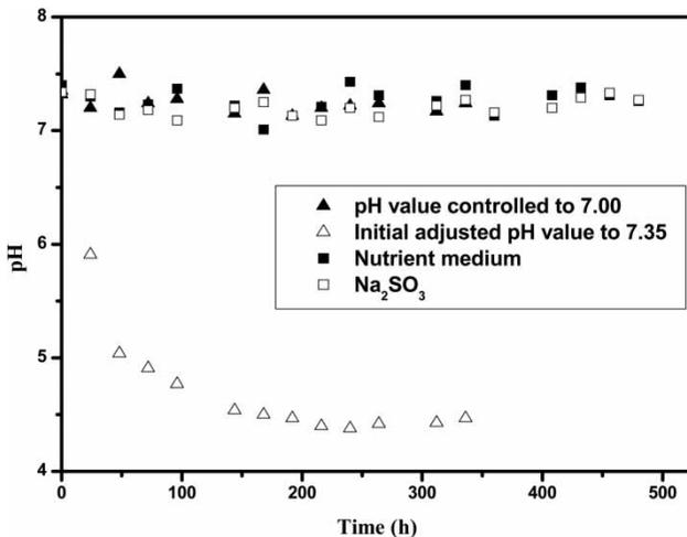
Figure 3 | pH value changes during anaerobic fermentation.
