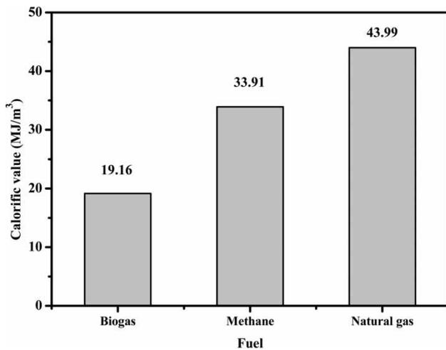
Figure 7 | Calorific values of different fuel gases.
