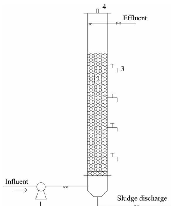
**Figure 1** | Schematic diagram of anaerobic continuous upflow biofilm reactor: (1) peristaltic pump; (2) ceramsite; (3) sampling port; (4) gas vent.
