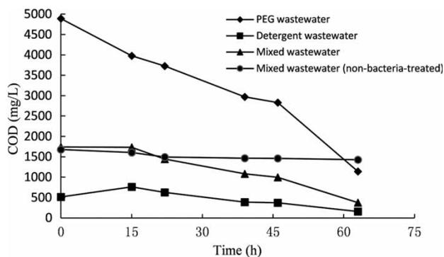
**Figure 3** | Small-scale test for COD removal performance after field bioaugmentation treatment of wastewater.
