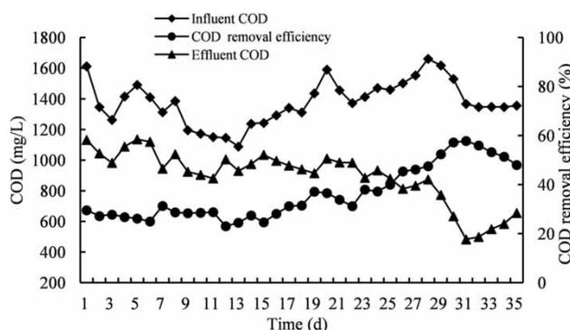
**Figure 2** | COD removal performance using previous wastewater treatment process without bioaugmentation.
