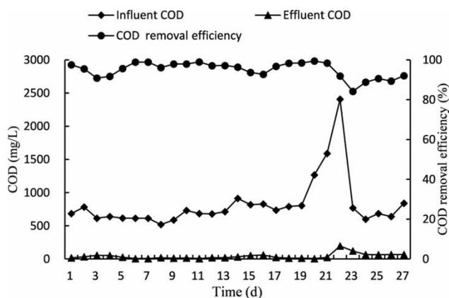
Figure 5 | Long-term COD removal performance of the bioaugmentation system.
