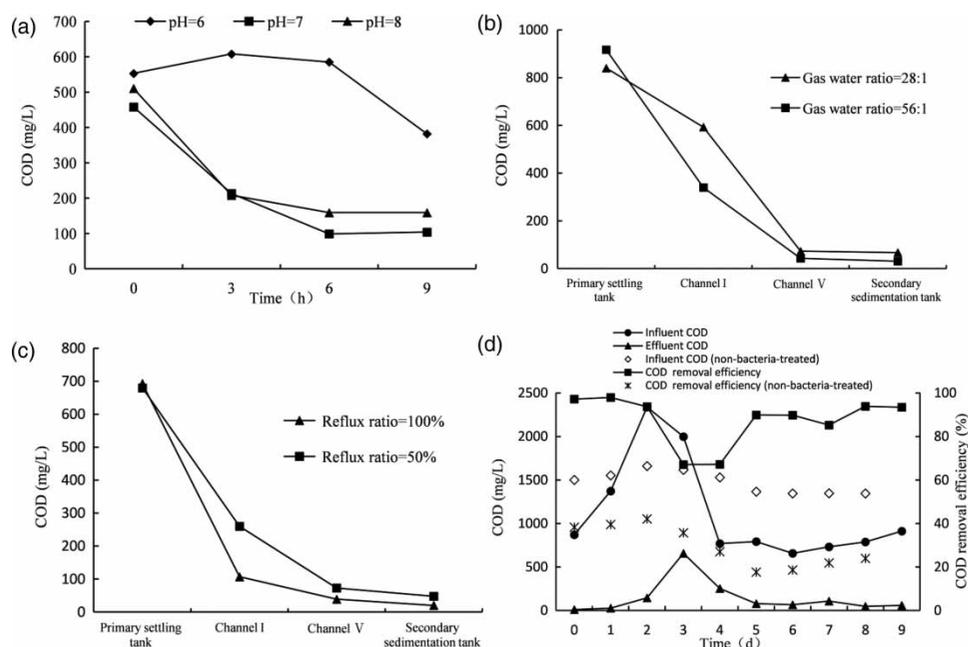
Figure 4 | Effect of pH on COD removal (a), gas–water ratio on COD removal (b), reflux ratio on COD removal (c), and shock load on COD removal (d) in the bioaugmentation system.
