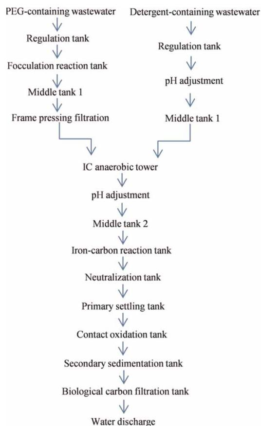
Figure 1 | Previous wastewater treatment process.
