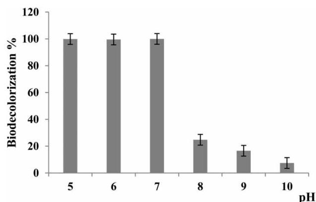
**Figure 3** | Effect of initial pH values on Congo Red biodecolorization efficiency.
