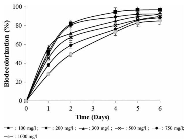
**Figure 2** | Effect of dye concentration on the biodecolorization efficiency of Congo Red under agitated conditions.
