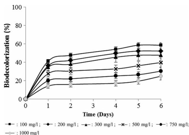
**Figure 1** | Effect of dye concentration on the biodecolorization efficiency of Congo Red under static conditions.
