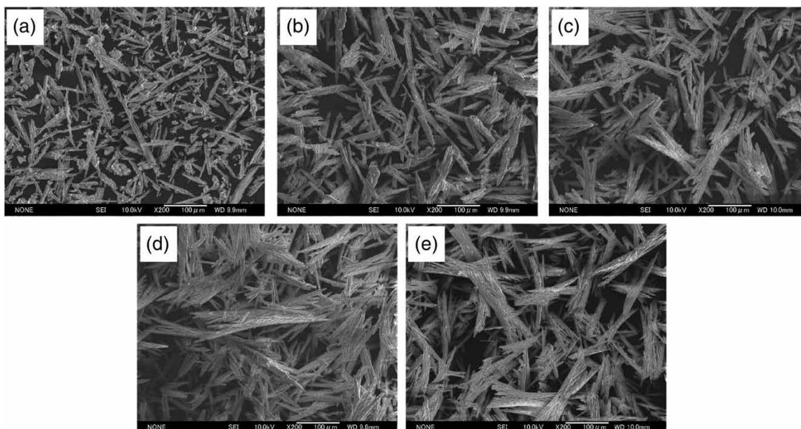
**Figure 2** | SEM images (200 $\times$ ) of precipitates from struvite precipitation in synthetic urine at different Mg:P molar ratios: (a) 0.5:1; (b) 1.0:1; (c) 1.2:1; (d) 1.5:1; and (e) 2.0:1.
