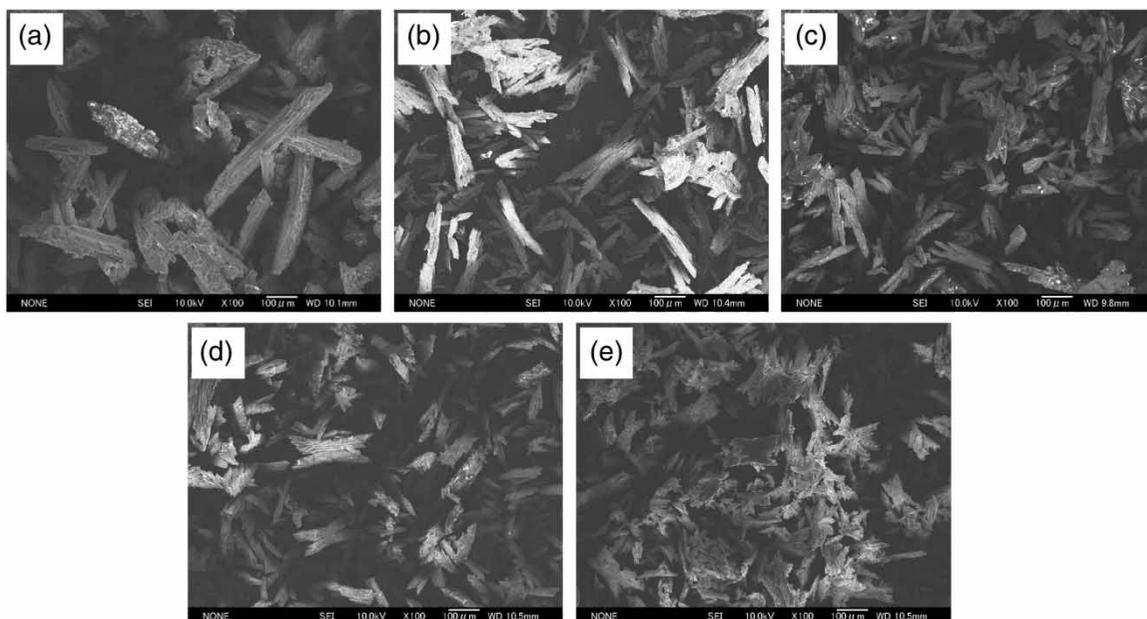
**Figure 3** | SEM images ( $\times 100$ ) of precipitates from struvite precipitation in human urine at different Mg:P molar ratios: (a) 0.6:1; (b) 1.0:1; (c) 1.2:1; (d) 1.5:1; and (e) 2.0:1.
