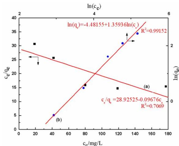
**Figure 8** | Adsorption isotherms of RhB onto nano-Ni<sub>2.33</sub>Fe. Fitting models: (a) Langmuir; (b) Freundlich.
