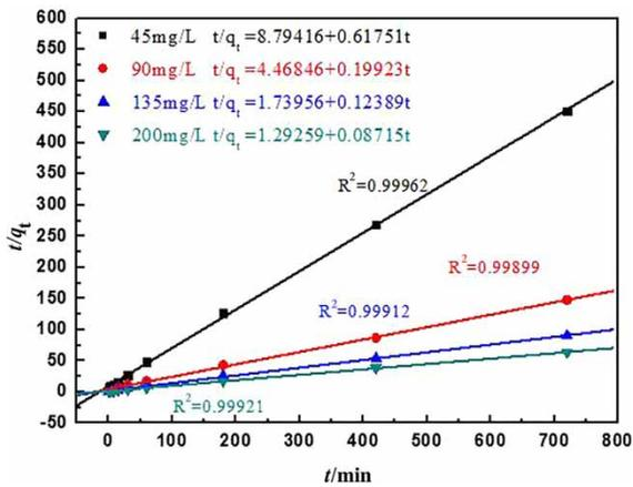
**Figure 6** | Plot of pseudo-second-order model at different concentrations of RhB for  $\text{Ni}_{2.33}\text{Fe}$  as adsorbent.
