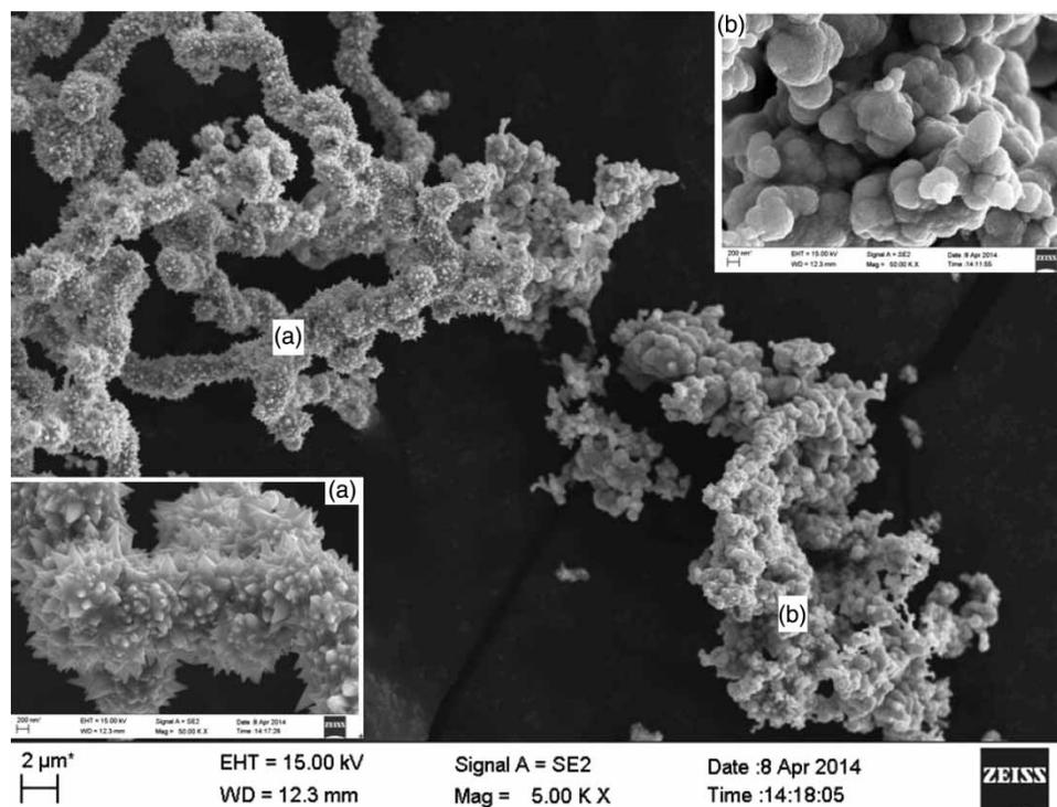
**Figure 2** | SEM images of  $\text{Ni}_{2.33}\text{Fe}$  (insert graph: magnified images for part (a) and part (b)).
