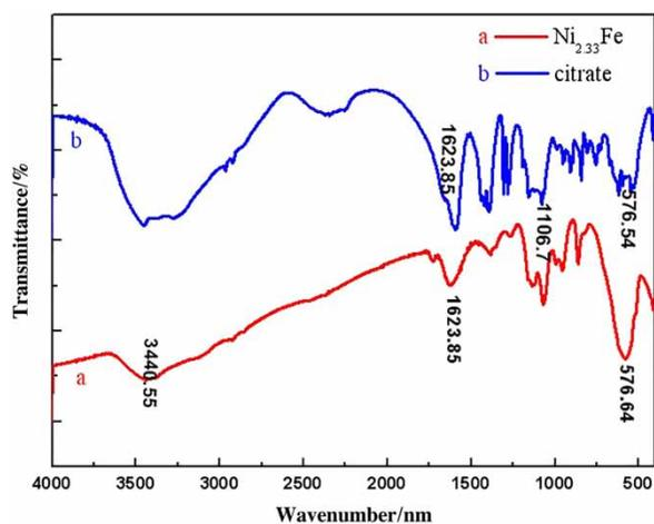
Figure 4 | IR spectra of nanoparticles  $\text{Ni}_{2.33}\text{Fe}$  and sodium citrate.
