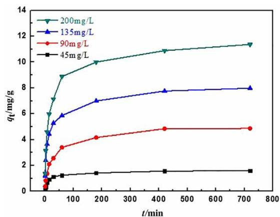
Figure 5 | Effect of contact time on the adsorption of RhB onto nanomagnetic  $\text{Ni}_{2.33}\text{Fe}$  particles at different RhB initial concentrations.
