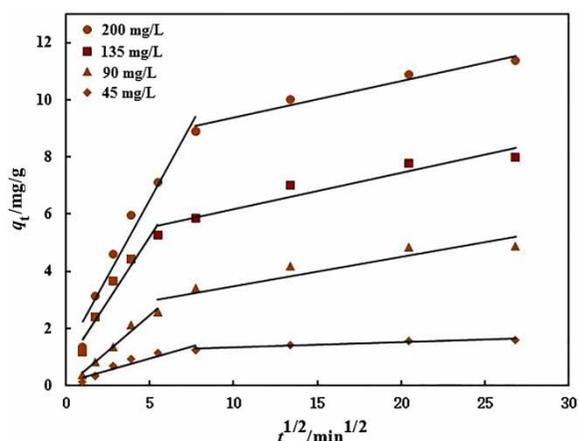
**Figure 7** | Weber-Morris intraparticle diffusion plots for RhB onto Ni<sub>2.33</sub>Fe at different concentrations of RhB.
