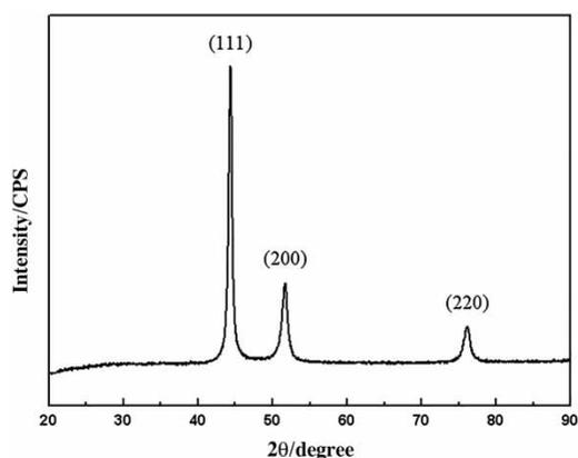
**Figure 1** | XRD pattern of  $\text{Ni}_{2.33}\text{Fe}$ .
