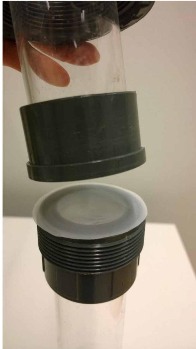
**Figure 3** | Filter is placed between the screw-on connectors.
