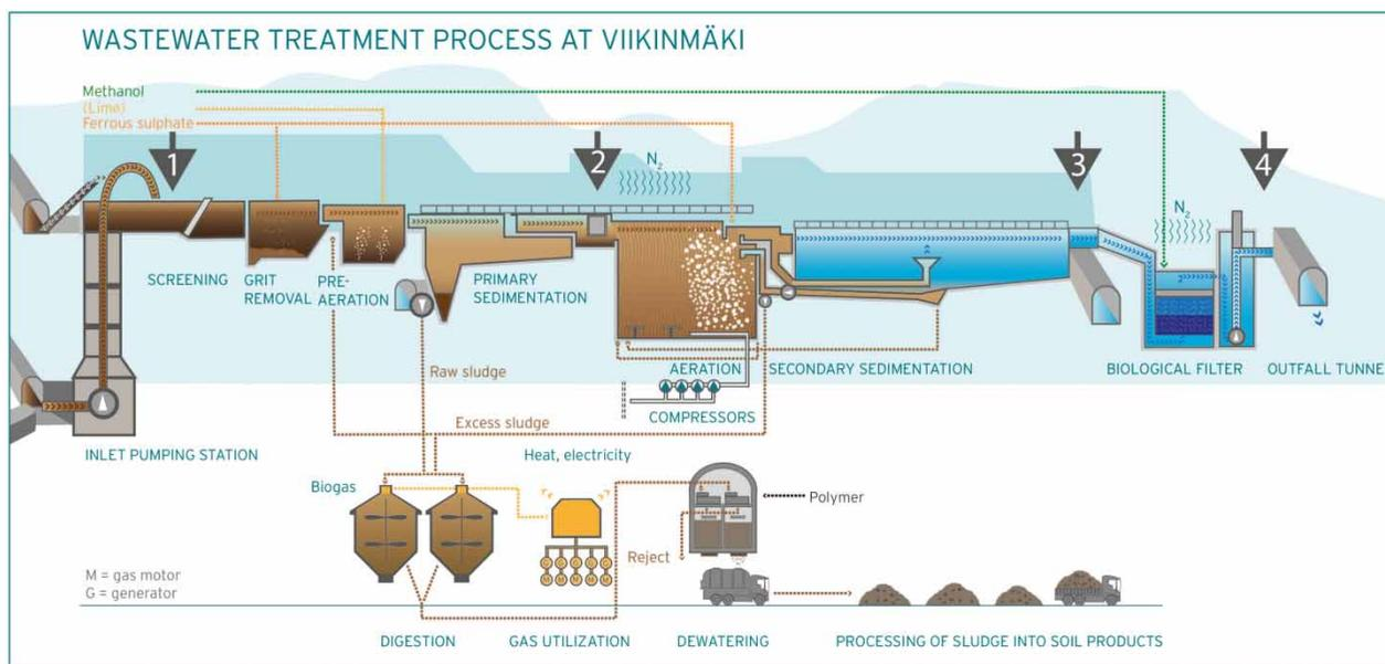
**Figure 1** | Wastewater treatment process at Viikinmäki. Sampling points are marked with arrows: influent (1), after the primary sedimentation (2), after the secondary sedimentation (3) and after the DN-post-filtration unit (4).
