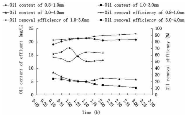
**Figure 1** | Coarse-graining effects with different ceramic padding sizes.
