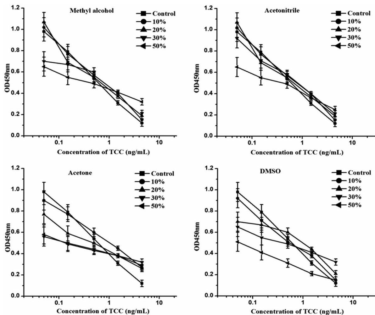
Figure 4 | Influence of different organic solution, methyl alcohol, acetonitrile, acetone and DMSO, on the performance of assay. Results are the means of three independent experiments.
