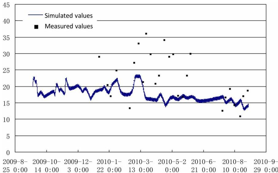
Figure 10 | Simulated and measured COD concentration of Jiangcungang section (mg/L).
