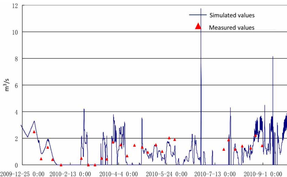
Figure 6 | Simulated and measured flow of Jiangcungang section ( $\text{m}^3/\text{s}$ ).
