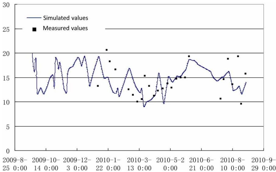
Figure 9 | Simulated and measured COD concentration of Wuchanggang section (mg/L).
