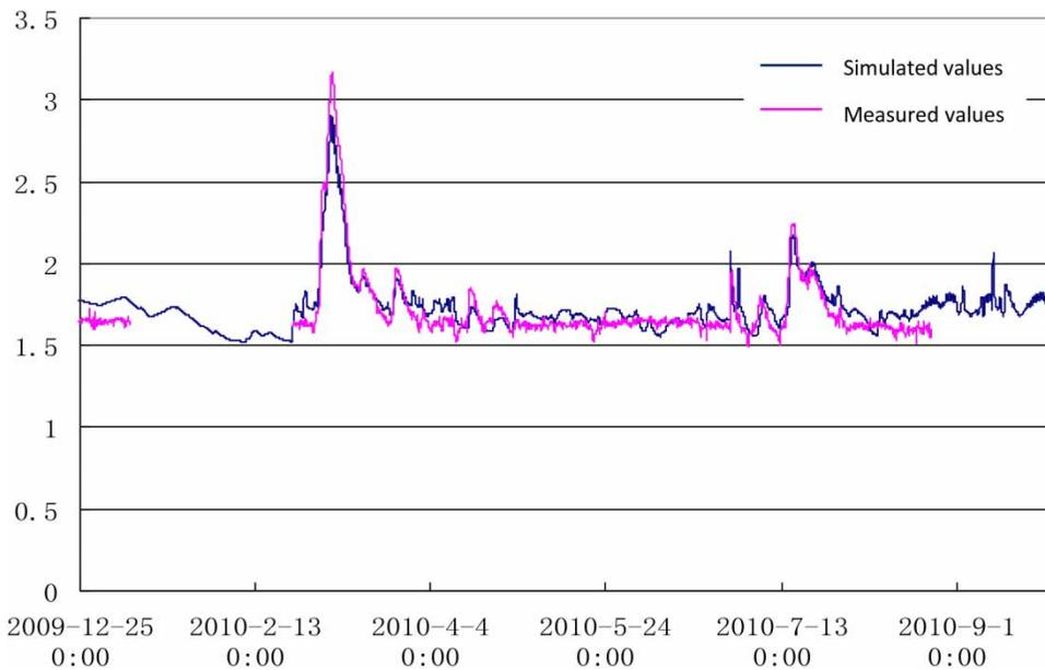
**Figure 7** | Simulated and measured water level of Zijiangang section (m).
