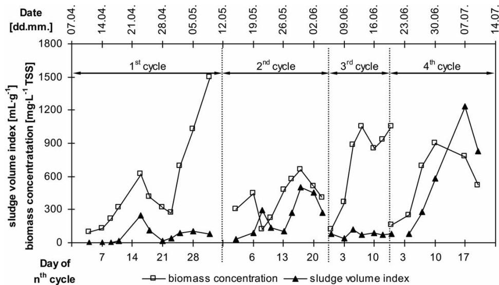
Figure 2 | Sludge volume index and biomass concentrations.
