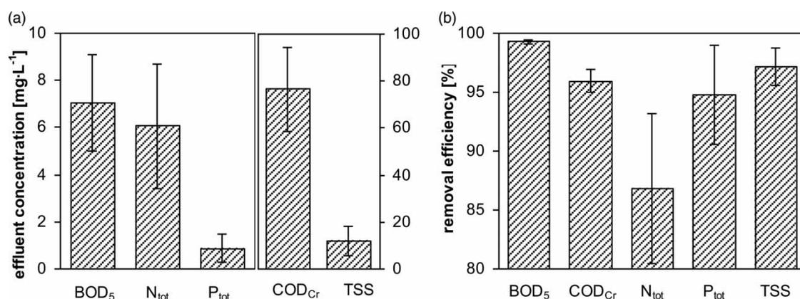
Figure 5 | Performance of microalgae-bacteria biomass: (a) treated wastewater concentrations; (b) removal efficiencies. Error bars represent standard deviation.
