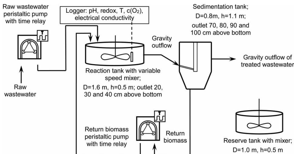
Figure 1 | Schematic of the pilot plant.
