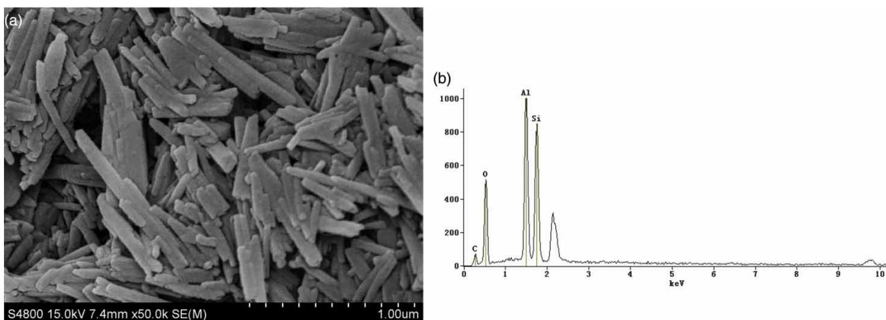
Figure 4 | SEM-EDX images of N-doped ZnO/HNTs: (a) SEM; (b) EDX.
