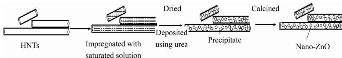
Figure 1 | Preparation illustration of N-doped ZnO/HNTs.
