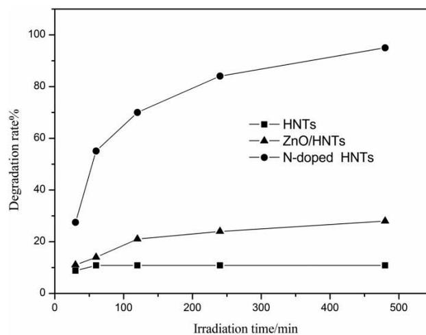
Figure 7 | The degradation rate of MO for HNTs, ZnO/HNTs and N-doped ZnO/HNTs.
