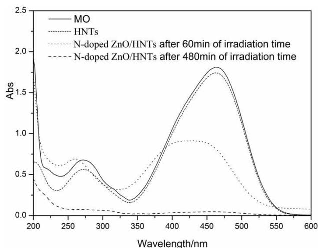
**Figure 8** | UV-vis absorption spectra of degradation of MO over HNTs and N-doped ZnO/HNTs.
