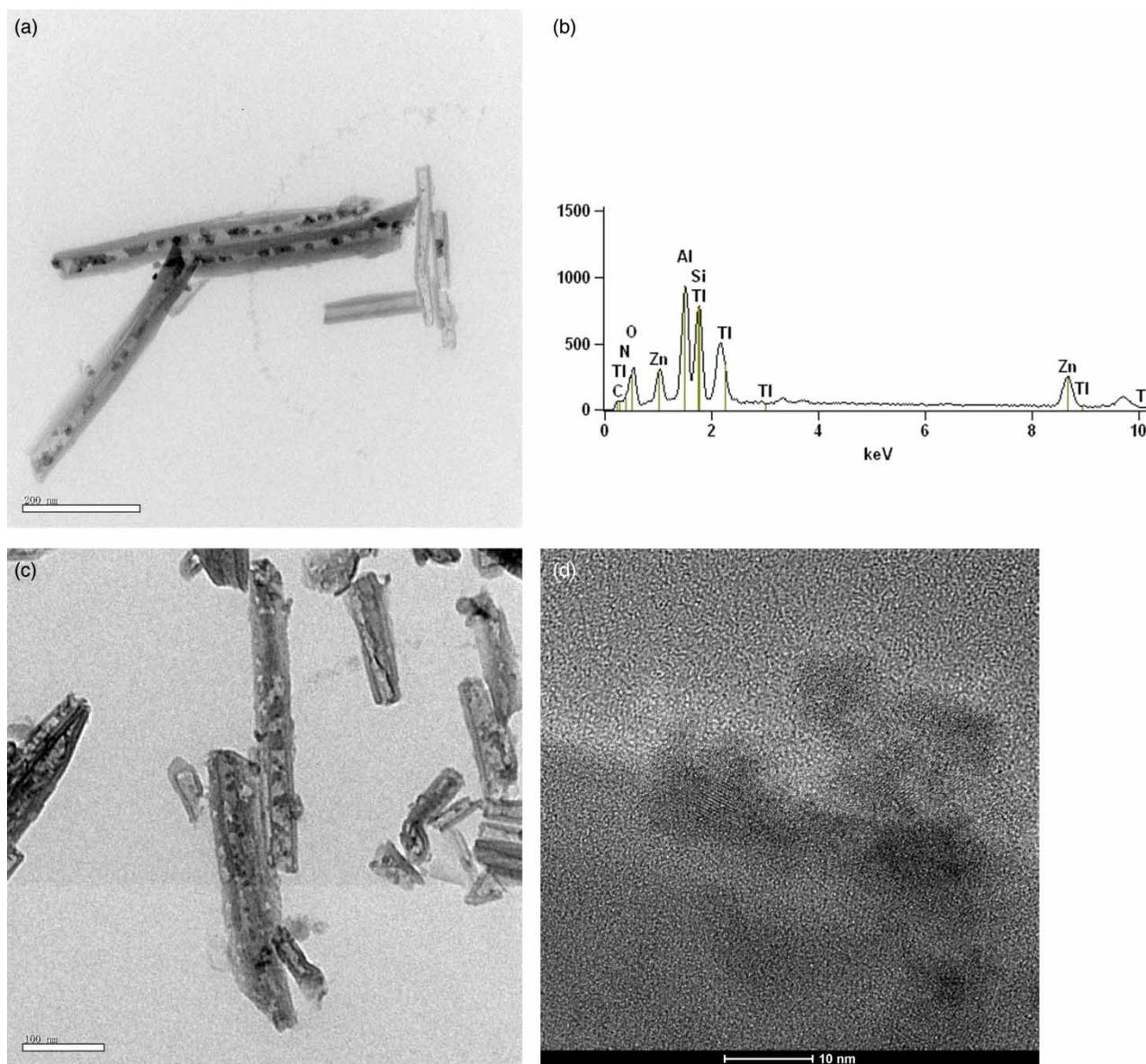
**Figure 3** | TEM-EDX images of N-doped ZnO/HNTs: (a) TEM; (b) EDX; (c) and (d) higher magnification.
