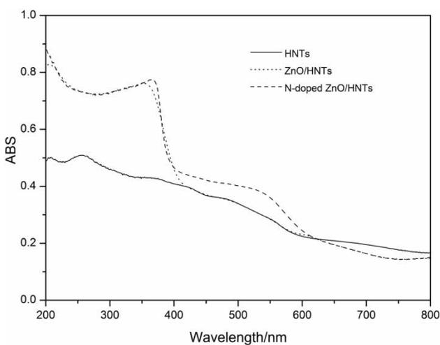
Figure 6 | UV-vis spectra of HNTs, ZnO/HNTs and N-doped ZnO/HNTs.
