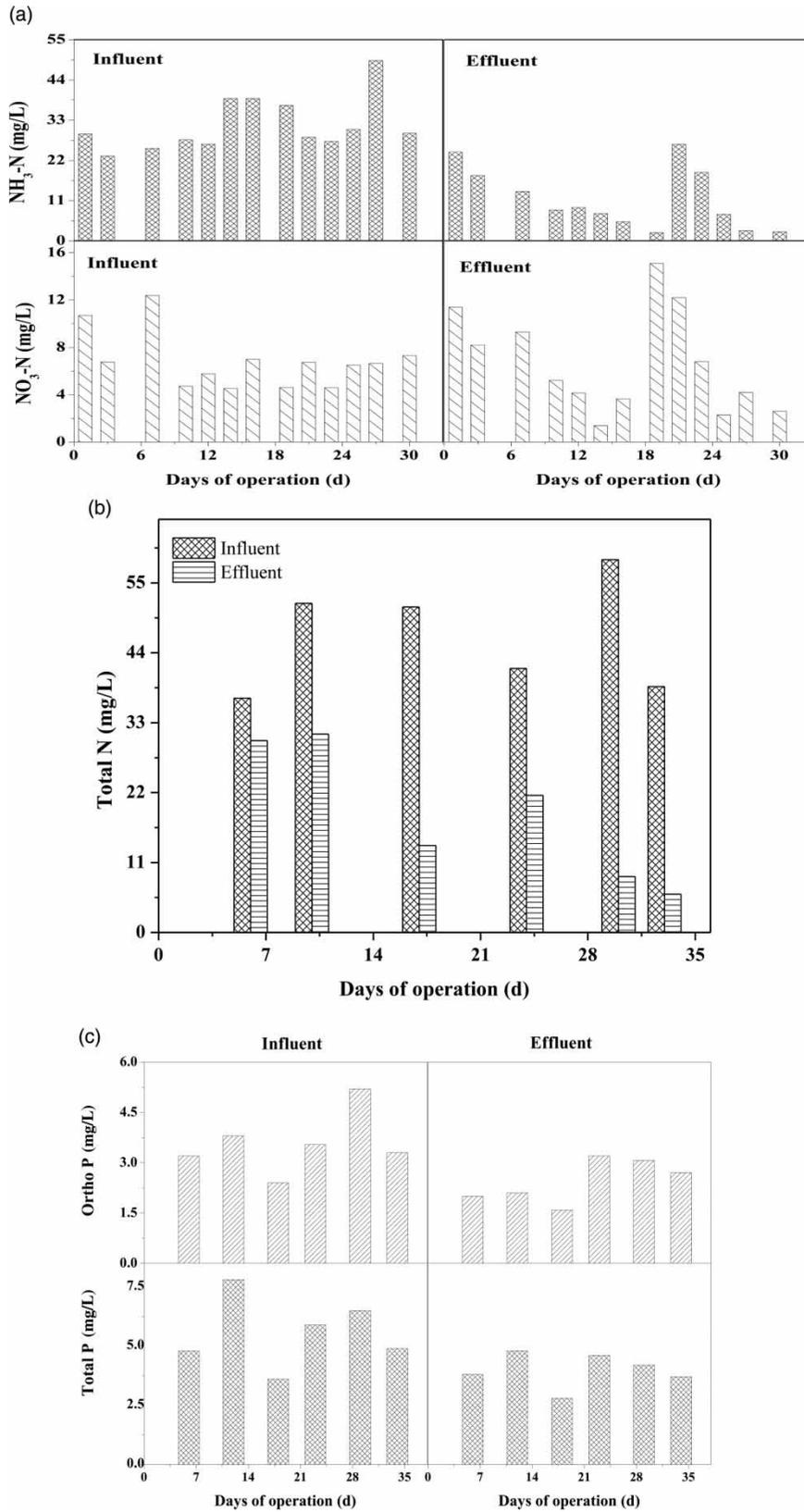
**Figure 4** | Influent and effluent concentrations of (a)  $\text{NH}_3\text{-N}$  and  $\text{NO}_3\text{-N}$ , (b) TN, and (c) OP and TP throughout the study period.
