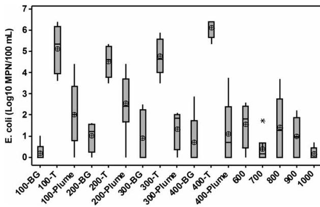
**Figure 2** | *E. coli* concentrations for sites served by onsite wastewater treatment systems (100–400) and municipal wastewater treatment systems (600–1000). Groundwater up-gradient from the onsite wastewater systems (BG), septic tanks (T), groundwater down-gradient from the onsite wastewater systems (Plume) are displayed.
