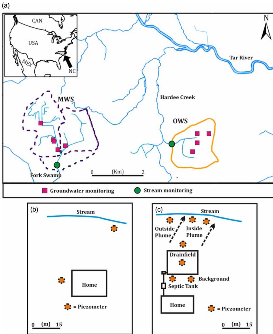
**Figure 1** | (a) Groundwater and stream monitoring sites in two watersheds within the coastal plain of North Carolina. One watershed was served by onsite wastewater systems (OWS) and the other by a municipal wastewater treatment sewer system (MWS). (b) Two or three piezometers were installed at each of the five MWS sites. (c) Networks of piezometers were installed up-gradient and down-gradient of onsite wastewater systems at four sites.
