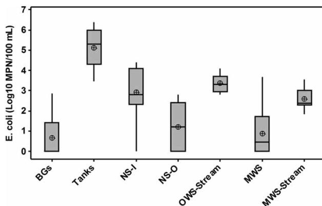
**Figure 3** | The combined  $\log_{10}$  of *E. coli* concentration data for all sampling locations including groundwater up-gradient from the onsite wastewater systems (BGS), septic tanks (Tanks), groundwater within the flow path of the systems and near the stream (NS-I) and groundwater outside the flow path of the systems and near the stream (NS-O), and the streams draining the onsite system watershed (OWS-Stream) and municipal wastewater system watershed (MWS-Stream).
