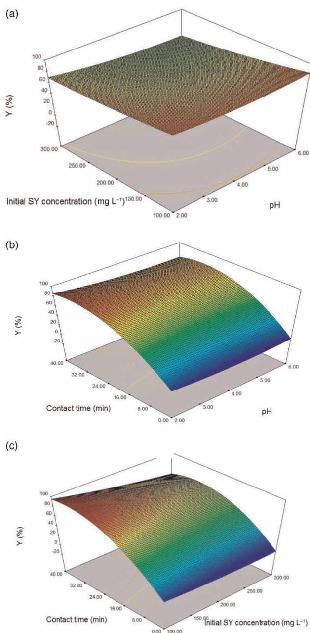
**Figure 4** | Response surface plots (3D) showing the effects of (a) pH and initial dye concentration, (b) pH and contact time, (c) contact time and initial dye concentration, and their influence on adsorption rate for removal of SY.
