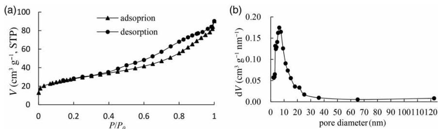
Figure 3 | (a)  $\text{N}_2$  adsorption/desorption isotherm of DE@C and (b) BJH pore size distribution. (STP: standard temperature and pressure).
