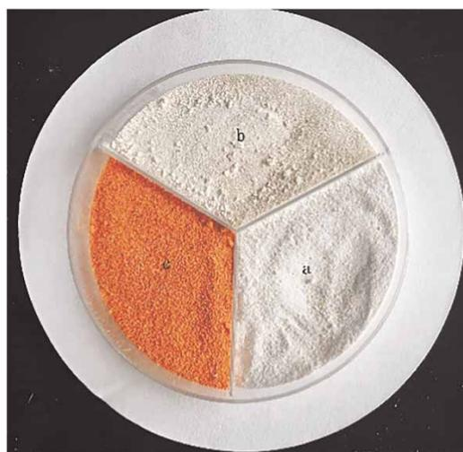
**Figure 1** | (a) Image of raw diatomite. (b) Image of diatomite earth@chitosan. (c) Image of diatomite earth@chitosan after adsorption.
