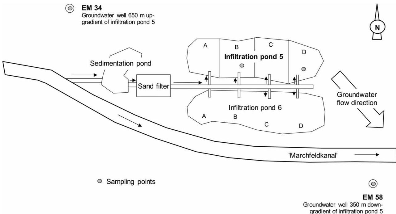
Figure 1 | Schematic illustration of the artificial recharge plant Stallingerfeld at Deutsch-Wagram, Austria.
