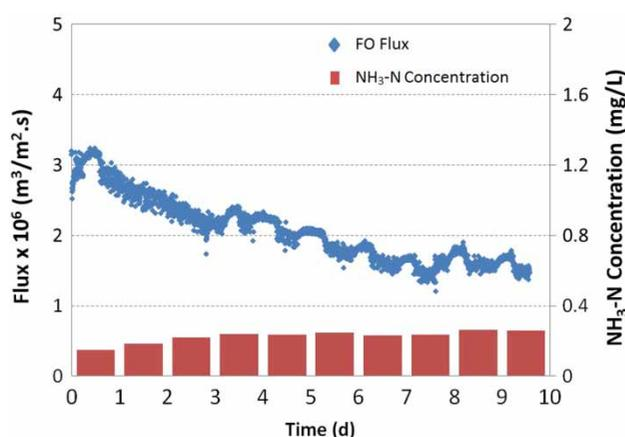
Figure 5 | Flux and  $\text{NH}_3\text{-N}$  concentrations in FO membrane durability test.
