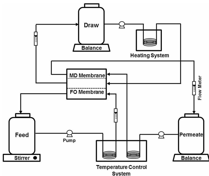
**Figure 1** | Schematic diagram of the integrated FO-MD membrane system.
