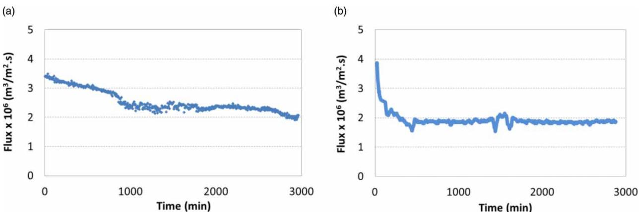
Figure 2 | Flux decline in (a) FO and (b) MD membrane systems.
