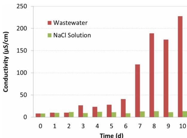
Figure 6 | Conductivity measurements in MD membrane durability test.
