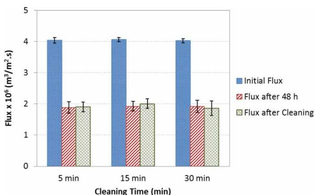
Figure 4 | Flux recoveries in MD membrane system.
