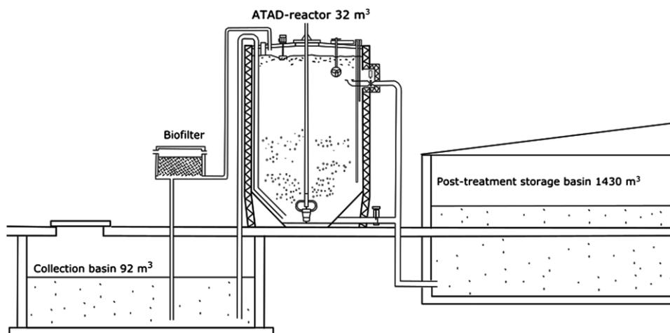
**Figure 1** | Schematic overview of the auto-thermal aerobic digestion plant comprising a 92 m<sup>3</sup> collection basin, a 32 m<sup>3</sup> reactor (height 7.5 m, Ø 3 m) (Alfa Laval Agri, Sweden) and a 1,430 m<sup>3</sup> covered post-treatment storage basin.
