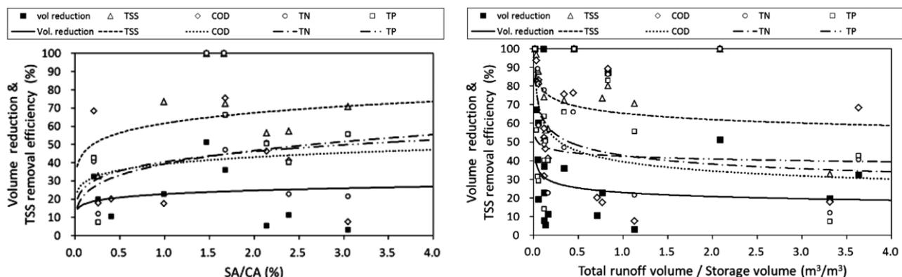
Figure 4 | Regression analysis for design of hybrid constructed wetland.
