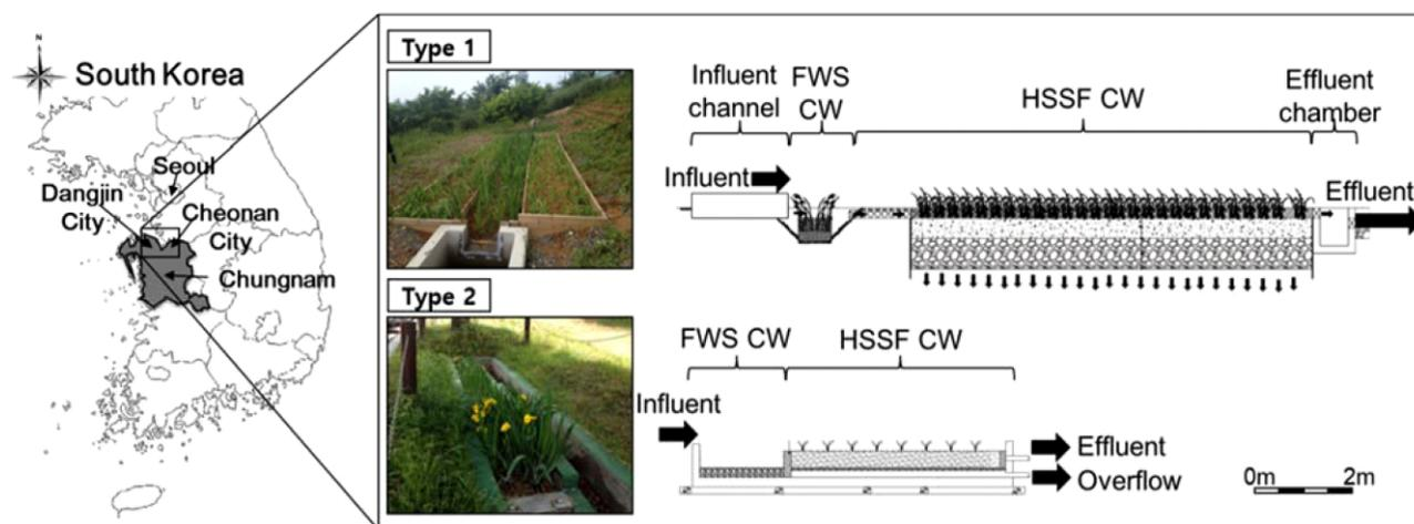
**Figure 1** | Location and schematic diagram of the hybrid CWS.
