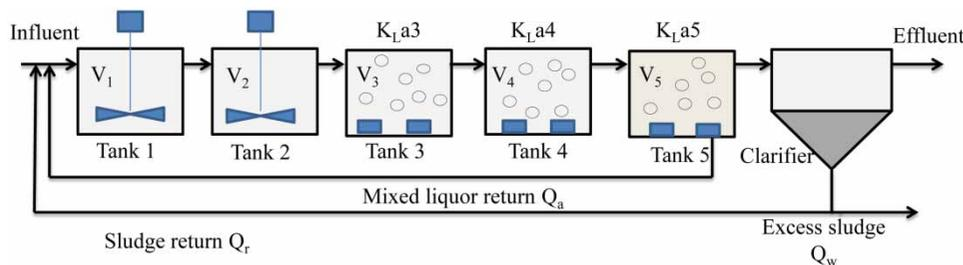
Figure 5 | Schematic representation of the BSM1.
