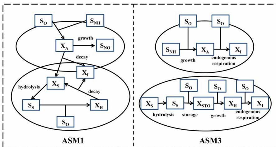
**Figure 2** | Substrate flows in ASM1 and ASM3. Source: redrawn from Gujer *et al.* (1999), Copyright IWA Publishing.
