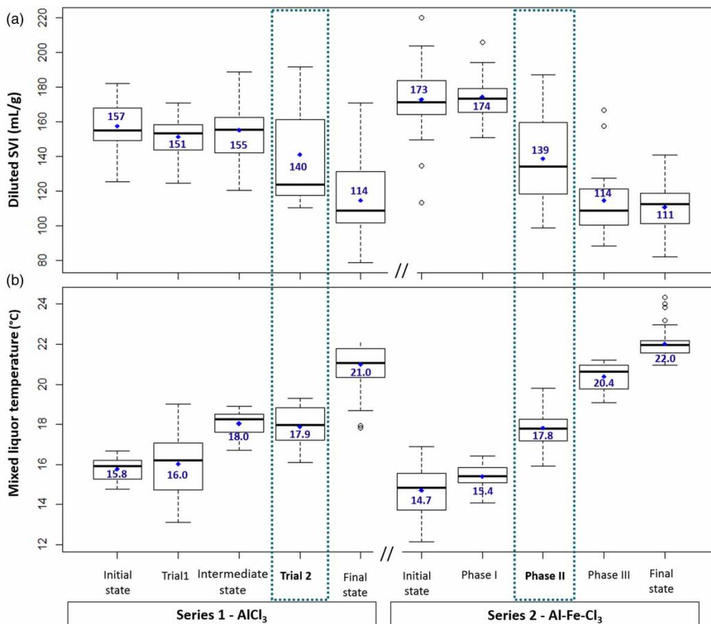
**Figure 3** | Box plot representation of DSVI (a) and temperature in C2 (b) during the different phases of the experiments. Circles correspond to the higher dosage in each series. The average value for each period is indicated by the diamond and the median by the thick line. Ends of the whiskers represent the lowest/highest data still within 1.5 interquartile range of the lower/upper quartile.
