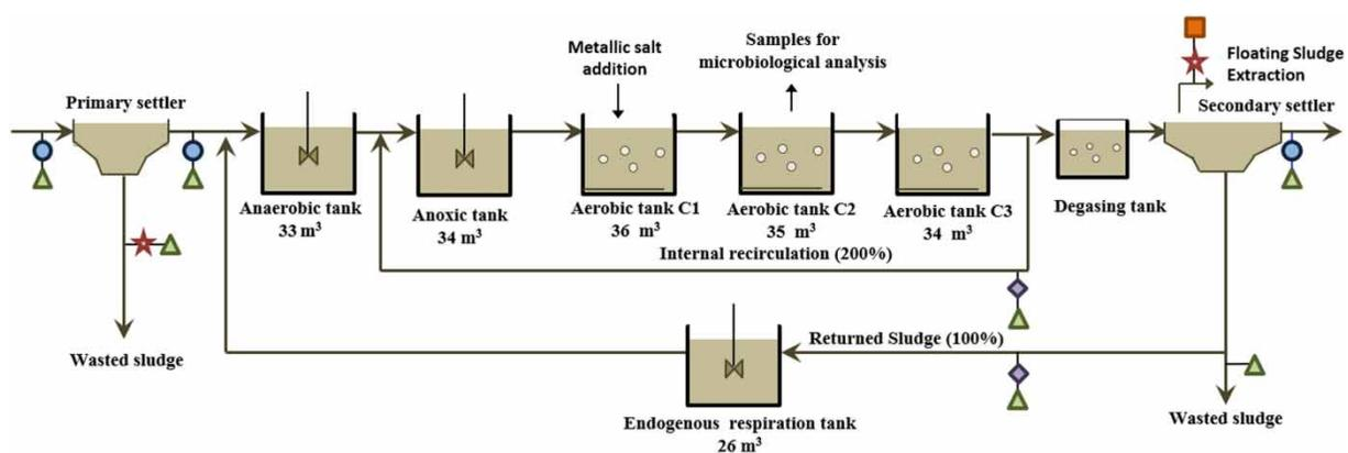
**Figure 1** | Scheme of the pilot plant: circle, 24 h flow proportional samples; diamond, daily grab samples; star, two samples a week; triangle, flowmeters; square, floating sludge extraction monitoring.
