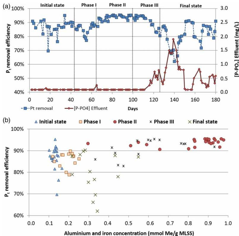
**Figure 2** | P-removal efficiency versus time (a) and as a function of the metallic salt concentration (b) for series 2.
