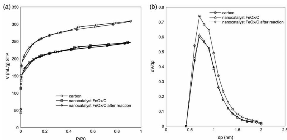
**Figure 4** | (a) Nitrogen sorption and desorption isotherms of the optimum nanocatalyst at 77 K; (b) microporous distribution.
