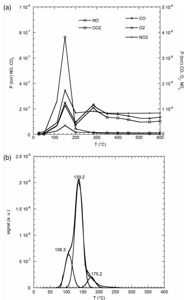
**Figure 3** | (a) Mass profile emissions from iron nitrate decomposition, supported with isopropyl alcohol on activated carbon. (b) Deconvolution of  $NO$  mass profile.
