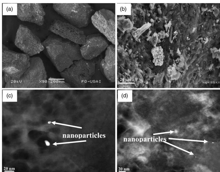
**Figure 5** | SEM micrographs of activated carbon or nanocatalyst support (a) and (b); TEM micrographs of the optimum nanocatalyst FeOx/C (c) and (d).
