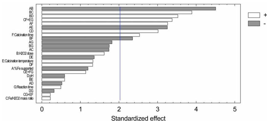
**Figure 1** | Standardized Pareto chart of the factor screening design for the Ae inactivation process using the heterogeneous Fenton-like reaction with FeOx/C nanocatalysts.
