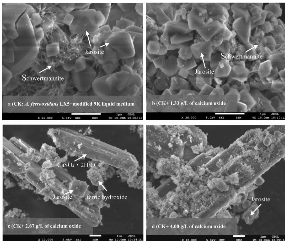
**Figure 5** | Effect of calcium oxide on SEM images of precipitates harvested from the modified 9 K liquid medium at 72 h with the addition of *A. ferrooxidans* LX5.
