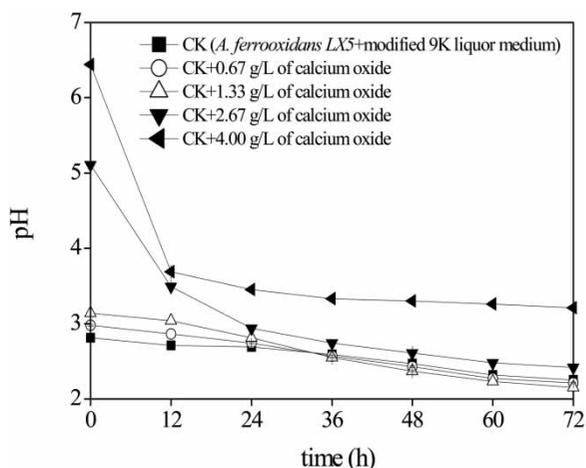
Figure 1 | Effect of calcium oxide on pH during ferrous ion oxidation in modified 9 K liquid medium with the addition of *A. ferrooxidans* LX5.
