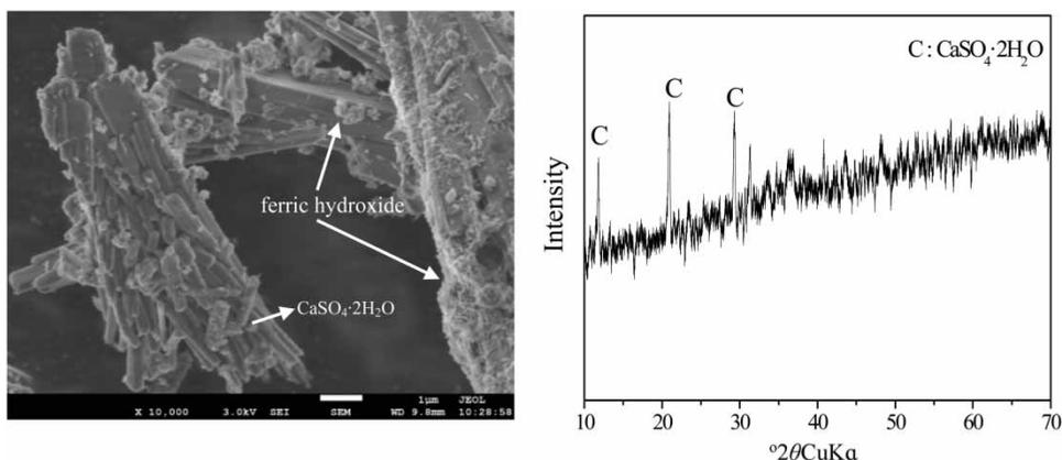
**Figure 6** | XRD pattern and SEM images of precipitates harvested from the modified 9 K liquid medium at 0 h with the addition of 1.33 g/L of calcium oxide.
