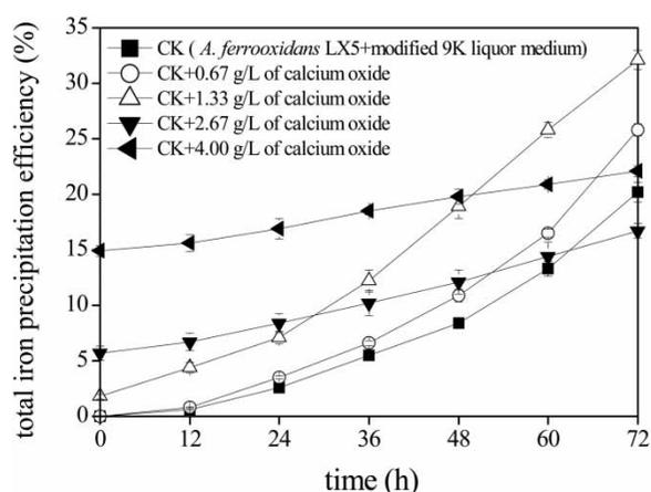
**Figure 3** | Effect of calcium oxide on the total iron precipitation efficiency during ferrous ion oxidation in modified 9 K liquid medium with the addition of *A. ferrooxidans* LX5.
