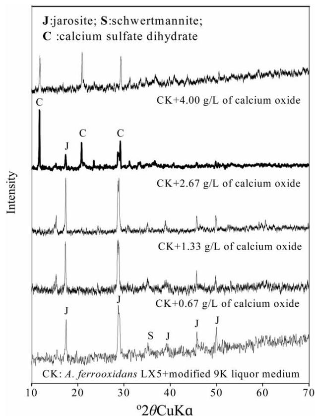
**Figure 4** | Effect of calcium oxide on XRD patterns of precipitates harvested from the modified 9 K liquid medium at 72 h with the addition of *A. ferrooxidans* LX5.
