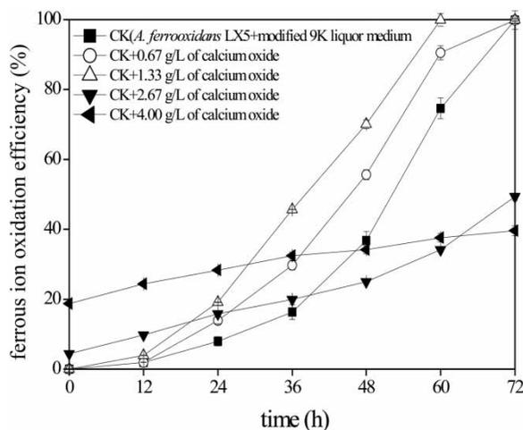
**Figure 2** | Effect of calcium oxide on the ferrous ion oxidation efficiency during ferrous ion oxidation in modified 9 K liquid medium with the addition of *A. ferrooxidans* LX5.
