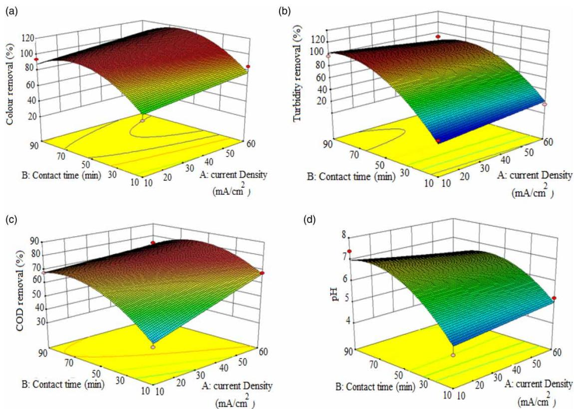
Figure 2 | 3D surface plots for colour (a), turbidity (b) and COD (c) removal efficiencies, and pH (d).
