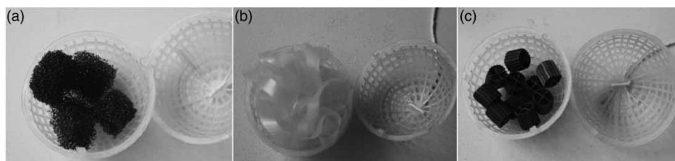
**Figure 3** | Three types of carriers: (a) porous carrier; (b) ribbon carrier; (c) ring carrier.
