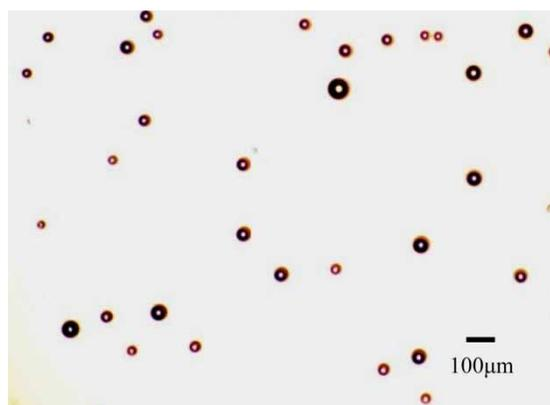
**Figure 2** | Observation of microbubbles generated by SPG membrane system in clean water.
