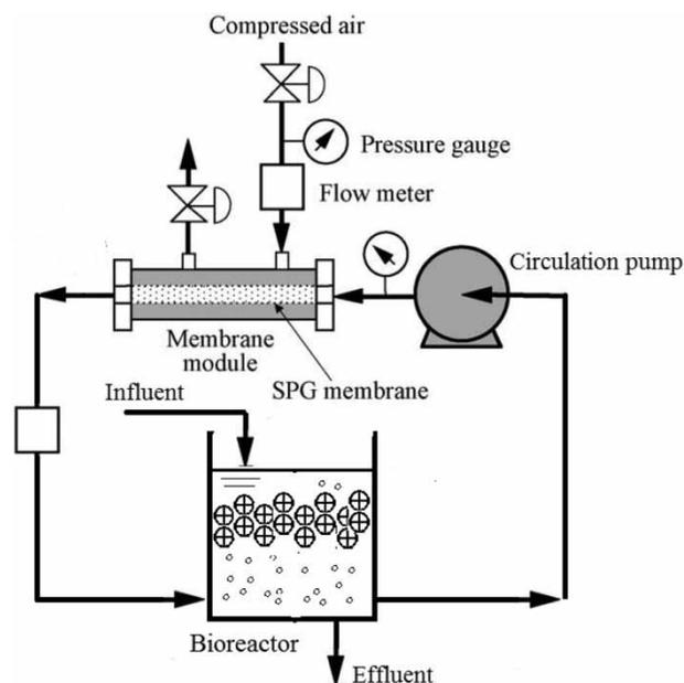
Figure 1 | Schematic diagram of the experimental apparatus.
