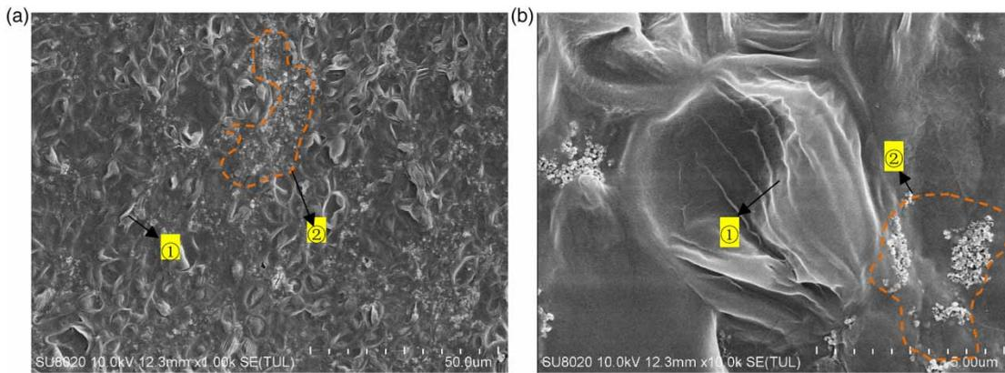
**Figure 2** | Surface structure of microalgal biofilm in LNS: (a) magnification of 1,000 times, (b) magnification of 10,000 times (① microalgae ② EPS secreted by microalgae).
