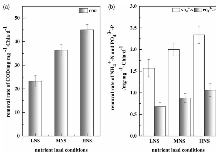
Figure 5 | Removal rates of nutrients in synthetic wastewater by algal biofilm in three nutrient loading conditions: (a) COD, (b) NH<sub>4</sub><sup>+</sup>-N and PO<sub>4</sub><sup>3-</sup>-P.
