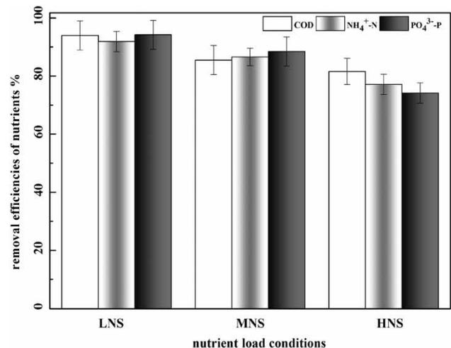
**Figure 4** | Removal efficiencies of nutrients in synthetic wastewater by algal biofilm in three nutrient loading conditions.
