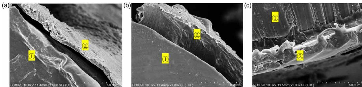
**Figure 3** | The thickness of microalgal biofilm in LNS (a), MNS (b) and HNS (c): ① carrier, ② microalgal biofilm.
