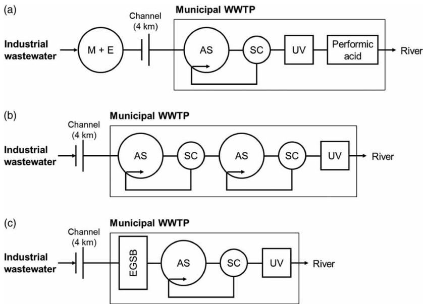
**Figure 1** | Layout of the WWTP in Warstein: (a) until July 2014, (b) at present (shut-down of the aerobic pre-treatment of the industrial wastewater), (c) near future (construction of an anaerobic pre-treatment for the industrial wastewater). AS: activated sludge, EGSB: expanded granular sludge bed reactor, M + E: mixing and equalization tank, SC: secondary clarifier, UV: ultraviolet disinfection.
