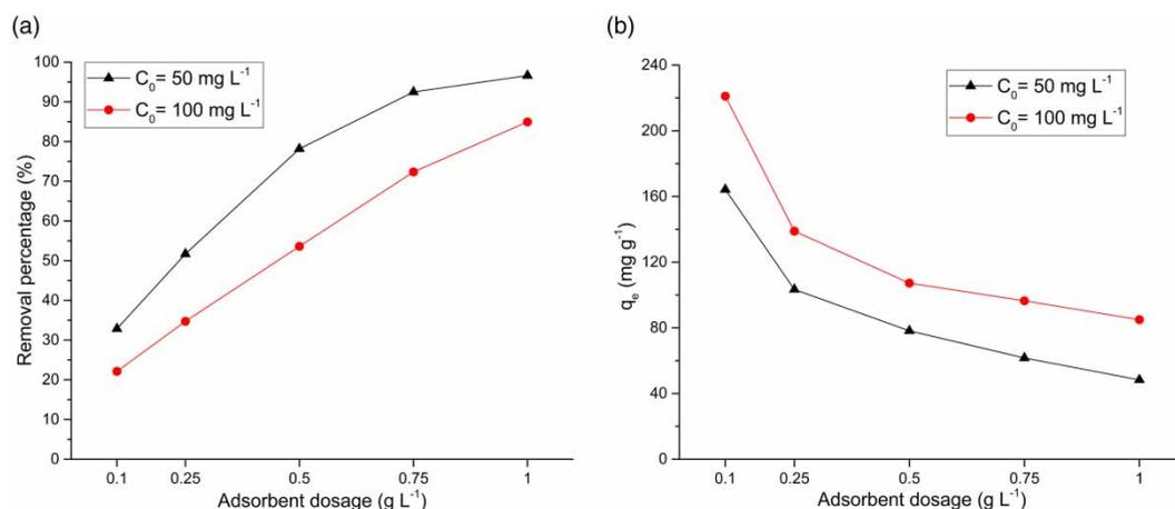
**Figure 5** | Effect of MWCNT dosage on the adsorption of TC: (a) represents removal percentage and (b) represents the amount of TC adsorbed. Conditions: natural pH; temperature 20 °C; contact time 4 h.
