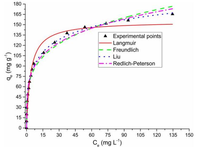
**Figure 8** | Isotherm curves for the adsorption of TC onto the MWCNT at 20 °C. Conditions: natural pH; adsorbent dosage 1 g L<sup>-1</sup>, contact time between the adsorbent and the adsorbate 4 h.**Table 5** | Isotherm parameters for the adsorption of TC onto the MWCNT adsorbent
