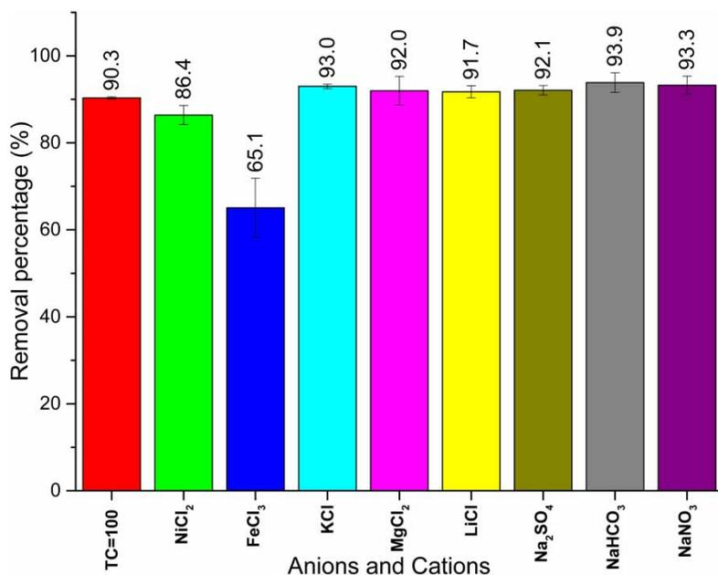
**Figure 6** | The adsorption of TC onto the MWCNT in the presence of 1 mM cations and anions, compared to control (initial TC 100 mg L<sup>-1</sup>). Error bars represent the SD of sample replicates. Conditions: natural pH; temperature 20 °C; contact time 4 h; adsorbent dosage 1 g L<sup>-1</sup>.
