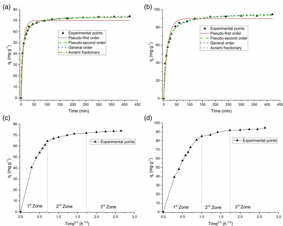
**Figure 7** | Kinetic curves for the adsorption of TC onto the MWCNT at 20 °C: (a)  $C_0 = 75$  mg L<sup>-1</sup>; (b)  $C_0 = 100$  mg L<sup>-1</sup>; (c) intra-particle diffusion for  $C_0 = 75$  mg L<sup>-1</sup>; (d) intra-particle diffusion for  $C_0 = 100$  mg L<sup>-1</sup>. Conditions: natural pH; adsorbent dosage 1 g L<sup>-1</sup>.
