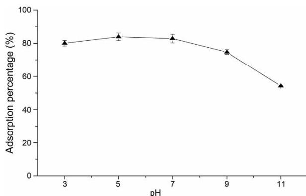
**Figure 4** | Effect of pH on the adsorption of TC onto MWCNT. Condition: temperature 20 °C; initial TC concentration 50 mg L<sup>-1</sup>; adsorbent dosage 0.5 g L<sup>-1</sup>.
