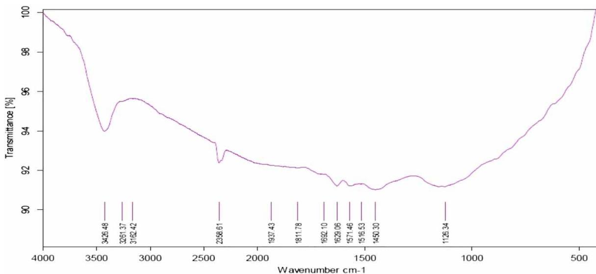
**Figure 1** | FTIR spectrum of the oxidized MWCNT.
