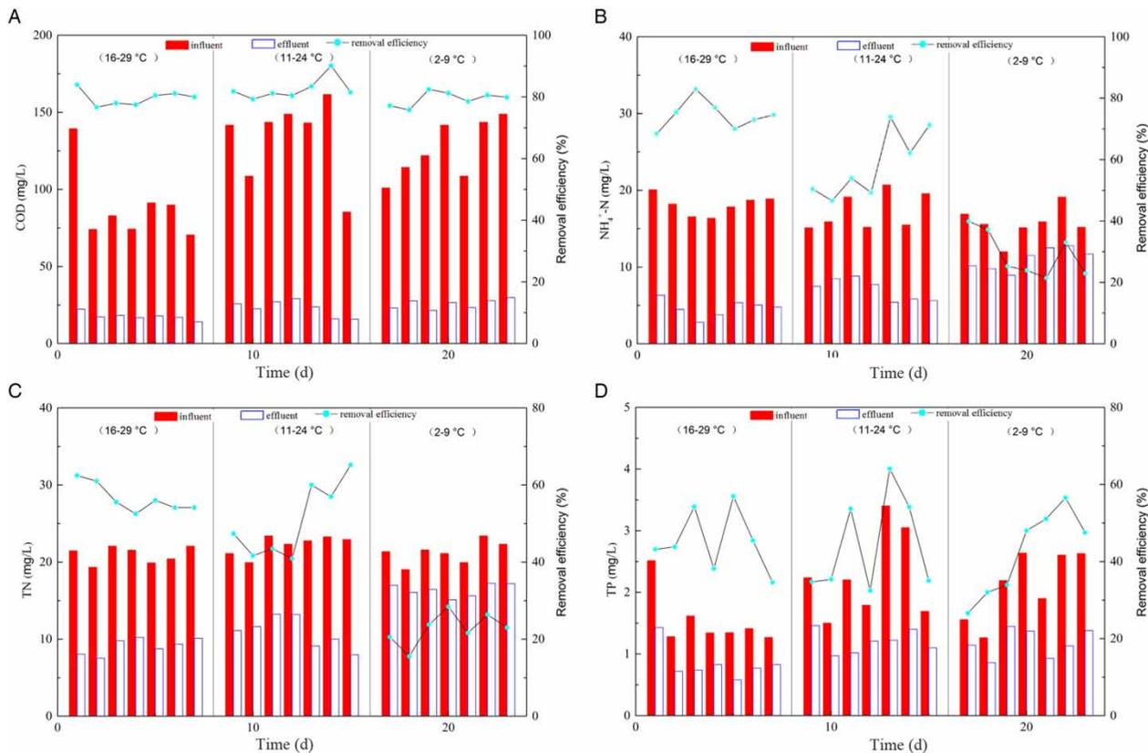
**Figure 3** | Impact of water temperature. A: Variations of COD; B: Variations of  $\text{NH}_4^+\text{-N}$ ; C: Variations of TN; D: Variations of TP.
