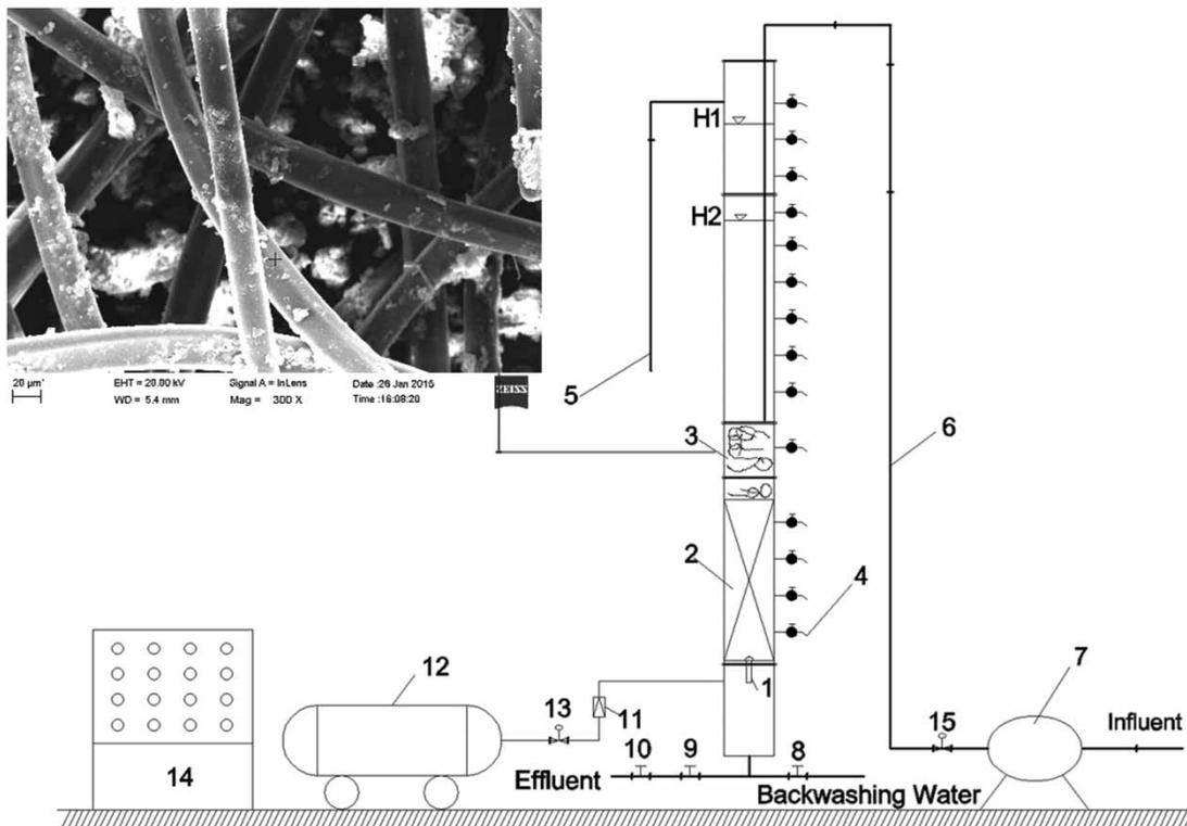
**Figure 1** | Sketch of SBBF. 1, long handle filter nozzle; 2, ceramsite filter media; 3, fibrous filler; 4, sampling point; 5, overflow pipe; 6, intake pipe; 7, pipeline pump; 8, backwashing water valve; 9, effluent regulating valve; 10, effluent electronic valve; 11, gas flowmeter; 12, air compressor; 13, intake electromagnetic valve; 14, control cabinet; 15, influent electromagnetic valve; H1, highest water level; H2, lowest water level.
