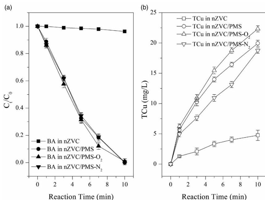
**Figure 5** | Variations of BA (a) and TCu (b) with reaction time in the nZVC/PMS process under the aerobic, anoxic, and anaerobic solutions. [BA]<sub>0</sub> = 20 μM, [PMS]<sub>0</sub> = 1 mM, [nZVC]<sub>0</sub> = 40 mg/L, O<sub>2</sub> flow rate = 0.3 L/min, N<sub>2</sub> flow rate = 0.8 L/min, pH<sub>0</sub> = 3.0.
