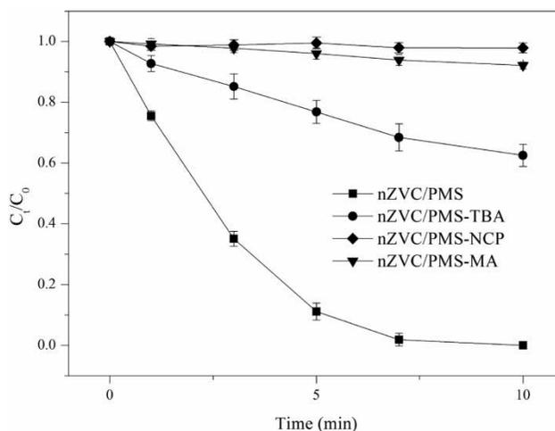
**Figure 2** | Inhibition of NCP, MA, and TBA on BA degradation in nZVC/PMS process.  $[\text{BA}]_0 = 20 \mu\text{M}$ ,  $[\text{PMS}]_0 = 1 \text{ mM}$ ,  $[\text{nZVC}]_0 = 40 \text{ mg/L}$ ,  $[\text{MA}]_0 = [\text{TBA}]_0 = 10 \text{ mM}$ ,  $[\text{NCP}]_0 = 1 \text{ mM}$ ,  $\text{pH}_0 = 3.0$ .
