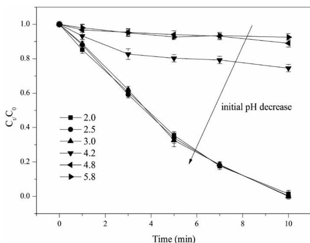
**Figure 7** | Effect of initial pH on BA degradation in the nZVC/PMS process.  $[BA]_0 = 20 \mu\text{M}$ ,  $[PMS]_0 = 1 \text{ mM}$ ,  $[nZVC]_0 = 40 \text{ mg/L}$ ,  $\text{pH}_0 = 2.0, 2.5, 3.0, 4.2, 4.8, \text{ and } 5.8$ .
