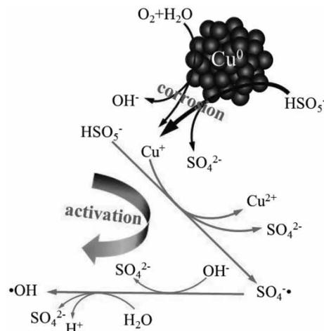
**Figure 6** | The mechanism of the nZVC/PMS process.
