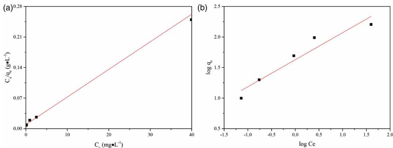
**Figure 5** | Isotherm plots for adsorption of MB onto LSP: (a) Langmuir and (b) Freundlich isotherm.
