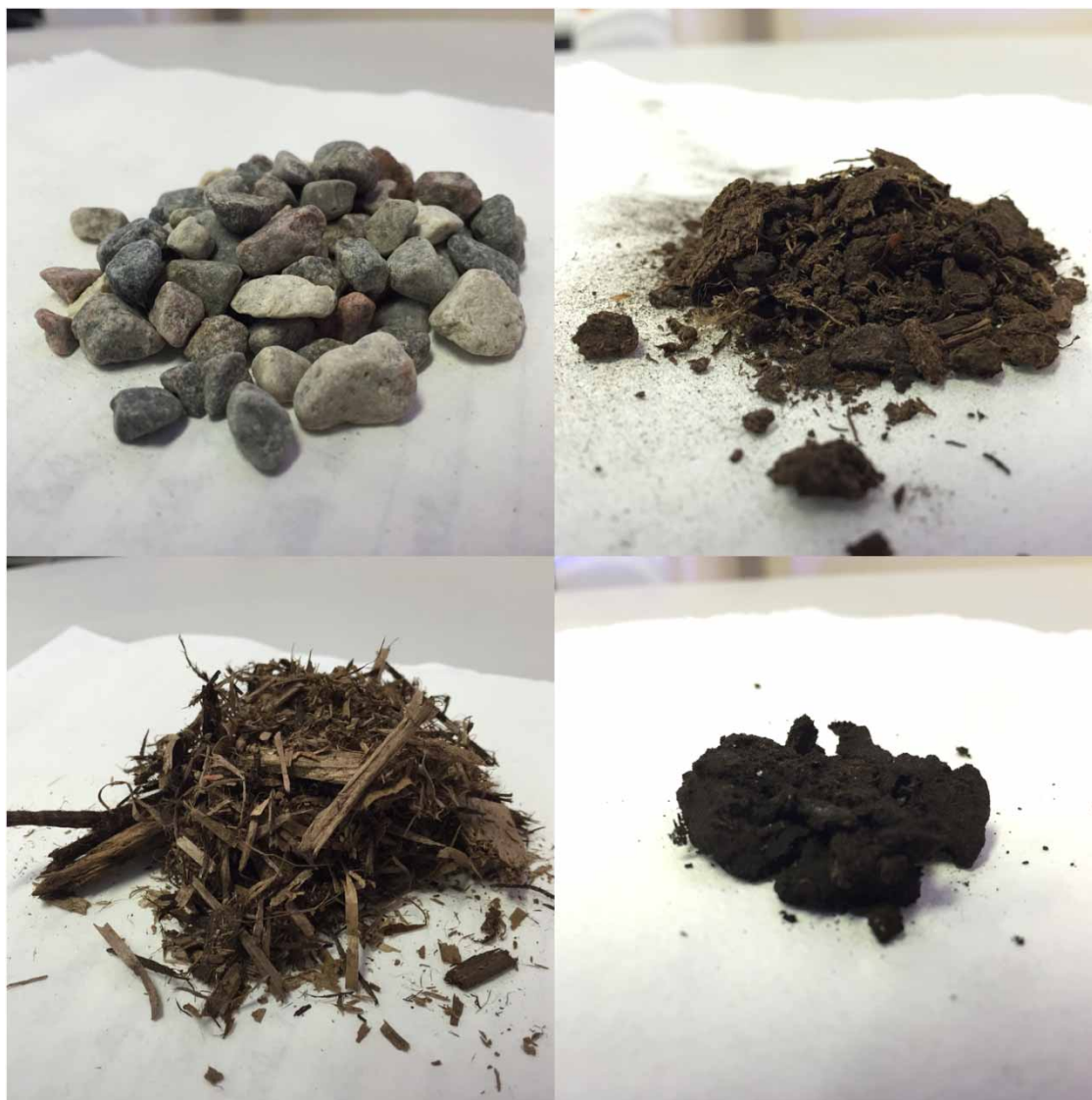
Figure 1 | Substrate material: gravel (top left), peat (top right), organic mulch (bottom left), topsoil (bottom right).
