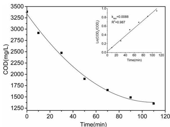
**Figure 1** | Trend of COD during the oxidation of guar gum solution by Fenton process. The inset panel shows its kinetic analysis assuming that COD follows a pseudo-first-order reaction. Dosing of  $\text{H}_2\text{O}_2$  10,000 mg/L,  $[\text{Fe}^{2+}] = 2,000$  mg/L, pH = 3, and  $T = 35^\circ\text{C}$ .
