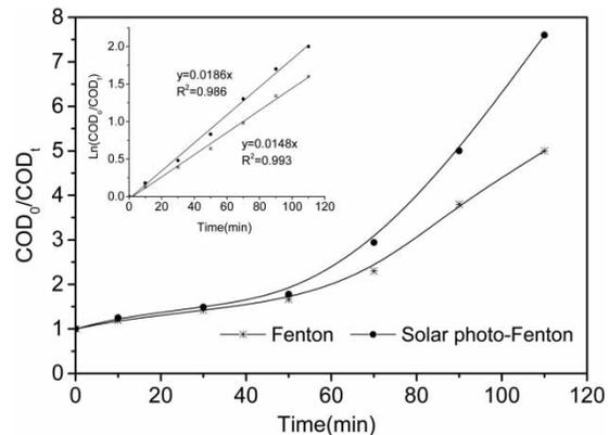
**Figure 11** | Effect of UV radiation on the kinetic abatement of COD during the treatment of wastewater ( $COD_0 = 413$  mg/L). The inset panel shows the fitting of the experimental data to a first-order reaction kinetic model concentration of  $H_2O_2$  10,000 mg/L,  $[Fe^{2+}]$  2,000 mg/L, pH = 3 and  $T$   $35^\circ C$ .
