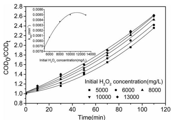
**Figure 2** | Effect of  $\text{H}_2\text{O}_2$  concentrations on the COD removal by the Fenton process. The inset panel shows  $k_{\text{app}}$  evolution at different dosing of  $\text{H}_2\text{O}_2$ .  $\text{COD}_0 = 3,386$  mg/L,  $[\text{Fe}^{2+}] = 2,000$  mg/L, pH = 3, and  $T = 35^\circ\text{C}$ .
