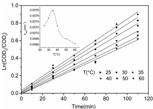
**Figure 9** | Plot of  $\ln(COD_0/COD_t)$  versus time at different temperatures.  $COD_0 = 3,386$  mg/L, concentration of  $H_2O_2$  10,000 mg/L,  $[Fe^{2+}] = 2,000$  mg/L and pH = 3.
