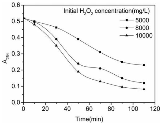
**Figure 3** | Temporal results of color evolution at 254 nm ( $A_{254}$ ). Effect of the concentration of  $H_2O_2$  upon color formation and abatement.  $COD_0 = 3,386$  mg/L,  $[Fe^{2+}] = 2,000$  mg/L,  $pH = 3$ , and  $T = 35$  °C.
