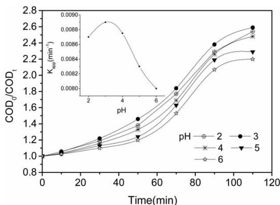
**Figure 7** | Effect of the initial pH on the COD removal by the Fenton process. The inset panel shows  $k_{\text{app}}$  evolution at different pH. Concentration of  $\text{H}_2\text{O}_2$  10,000 mg/L,  $[\text{Fe}^{2+}] = 2,000$  mg/L and  $T = 35^\circ\text{C}$ .
