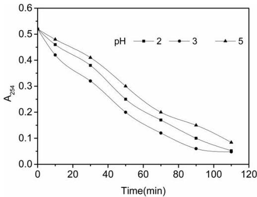
**Figure 8** | Temporal results of color evolution at 254 nm ( $A_{254}$ ). Effect of the initial pH upon color formation and abatement. Concentration of  $H_2O_2$  10,000 mg/L,  $[Fe^{2+}] = 2,000$  mg/L and  $T = 35^\circ C$ .
