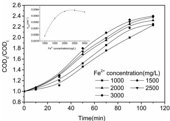
**Figure 4** | Effect of the initial concentration of  $Fe^{2+}$  on the COD removal by Fenton process. The inset panel shows  $k_{app}$  evolution at different  $Fe^{2+}$  concentration.  $COD_0 = 3,386$  mg/L, concentration of  $H_2O_2$  10,000 mg/L,  $pH = 3$ , and  $T = 35$  °C.
