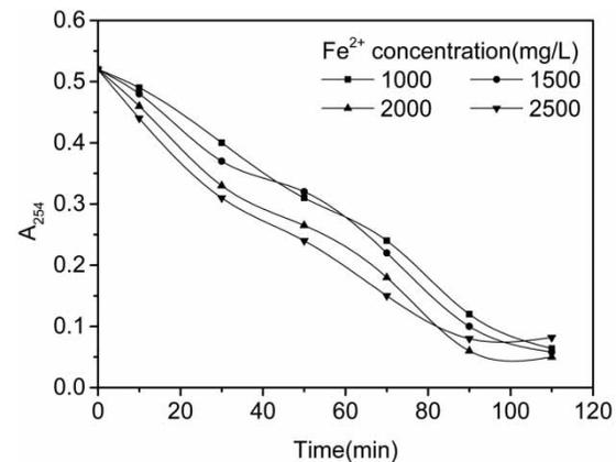
**Figure 5** | Temporal results of color evolution at 254 nm ( $A_{254}$ ). Effect of the initial concentration of ferrous ions upon color formation and abatement.  $COD_0 = 3,386$  mg/L, concentration of  $H_2O_2$  10,000 mg/L,  $pH = 3$ , and  $T = 35$  °C.
