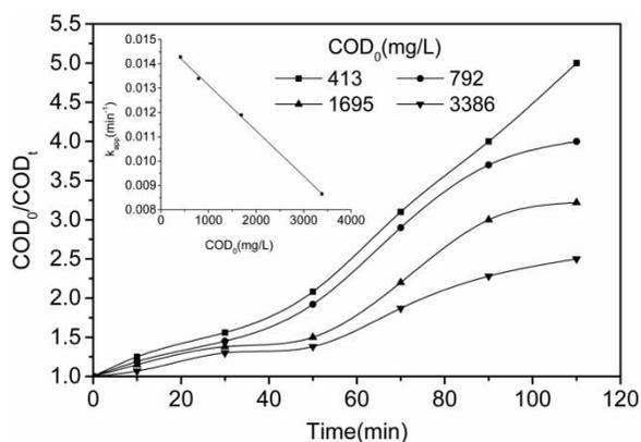
**Figure 6** | Effect of the initial concentration of guar gum on the COD removal by the Fenton process. The inset panel shows  $k_{\text{app}}$  evolution at different initial COD. Concentration of  $\text{H}_2\text{O}_2$  10,000 mg/L,  $[\text{Fe}^{2+}] = 2,000$  mg/L, pH = 3, and  $T = 35^\circ\text{C}$ .
