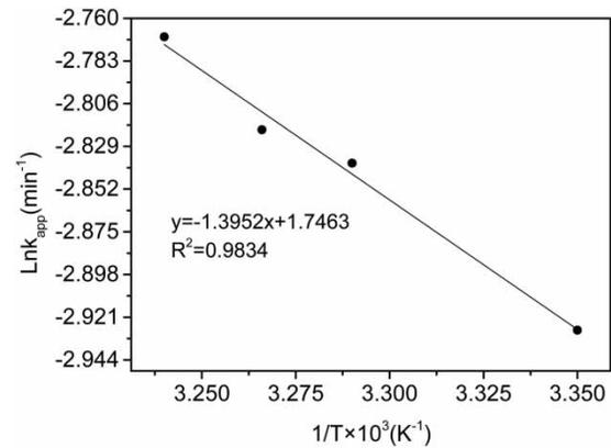
**Figure 10** | Plot of  $\ln k_{app}$  versus  $1/T$  for the degradation of guar gum by Fenton oxidation process.  $COD_0 = 3,386$  mg/L, concentration of  $H_2O_2$  10,000 mg/L,  $[Fe^{2+}] = 2,000$  mg/L and pH = 3.
