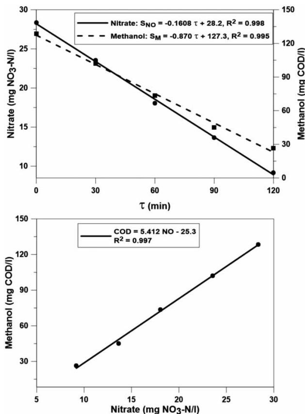
**Figure 1** | Results of the 2-hour DNR test on day 2 of the first run for the sludge taken from the aerobic decay reactor with a VSS of around 1,300 mg/L. (Top) Nitrate and methanol uptake rates, where the time axis is the same as in Equation (4). The NUR in this particular DNR test is 0.1608 mg  $\text{NO}_3\text{-N/L/min}$ . (Bottom) The ratio of COD/N, which is 5.412 in this particular test, resulting in the observed biomass yield coefficient of 0.47 by applying Equation (8).
