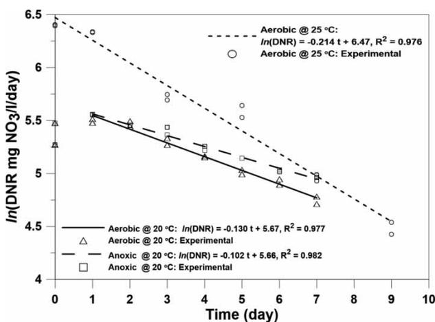
**Figure 2** | DNR reduction profile under aerobic and anoxic starvation conditions in the decay reactors at 20 °C for the first run, and under aerobic starvation conditions at 25 °C for the second run. The initial biomass VSS was 1,300 mg/L and 1,900 mg/L in each DNR test for the first and second run, respectively. Scatter symbols show duplicate DNR results for each DNR test. The coefficient of  $t$  in the linear regression model shows the value of the endogenous respiration rate.
