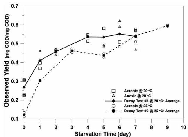
**Figure 3** | The observed biomass yield coefficients during 2-hour DNR test with respect to starvation-induced time. The solid and dashed lines connect the average observed biomass yield for the first and second run, respectively.
