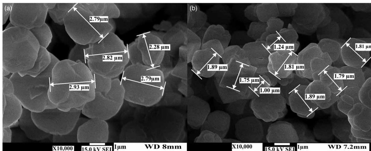
Figure 1 | SEM micrographs of (a) ZU and (b) ZN ( $\times 10,000$ ).
