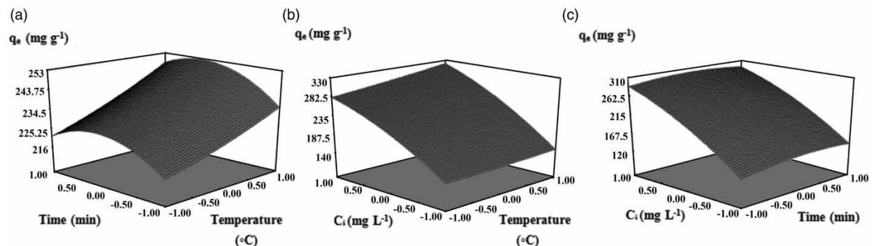
**Figure 4** | 3D response surface plots exhibiting the interactive effects of (a) temperature ( $x_1$ ) and time ( $x_2$ ), (b) temperature ( $x_1$ ) and initial concentration of Pb(II) ions ( $C_i$ ,  $x_3$ ), (c) initial concentration of Pb(II) ions ( $C_i$ ,  $x_3$ ) and time ( $x_2$ ), on adsorption capacity of ZN.
