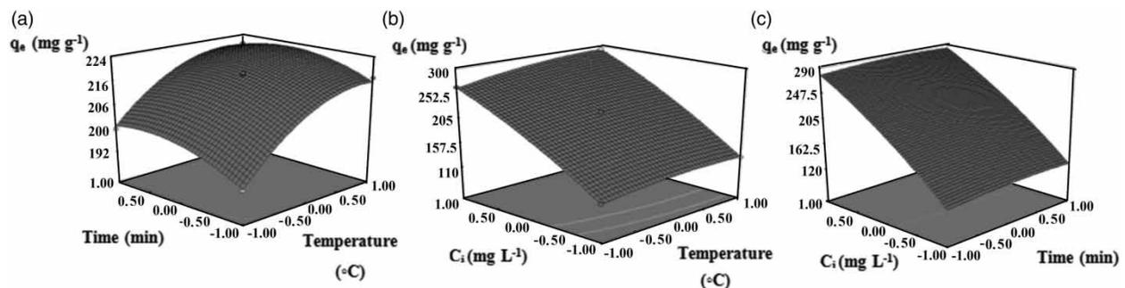
**Figure 3** | 3D response surface plots exhibiting the interactive effects of (a) temperature ( $x_1$ ) and time ( $x_2$ ), (b) temperature ( $x_1$ ) and initial concentration of Pb(II) ions ( $C_i$ ,  $x_3$ ), (c) initial concentration of Pb(II) ions ( $C_i$ ,  $x_3$ ) and time ( $x_2$ ), on adsorption capacity of ZU.
