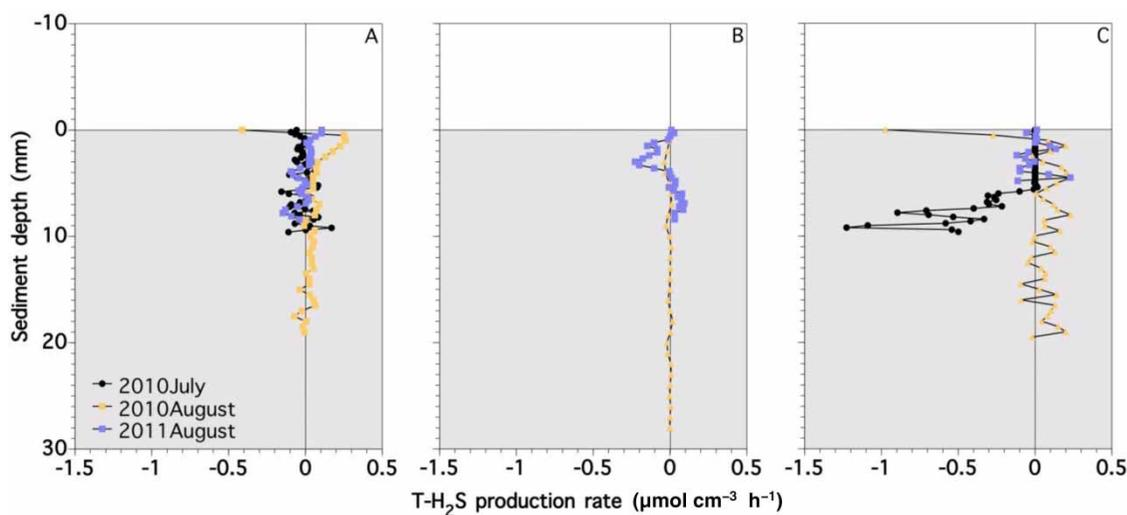
**Figure 3** | Vertical distribution and magnitude of the net volumetric T-H<sub>2</sub>S production rates ( $R(T-H_2S)$ ) in the sediment samples at Site 1 (a), Site 2 (b) and Site 3 (c). The rates were calculated based on the corresponding concentration profiles shown in Figure 2. Negative values indicate consumption. Zero on the vertical axis corresponds to the surface of the sediment.
