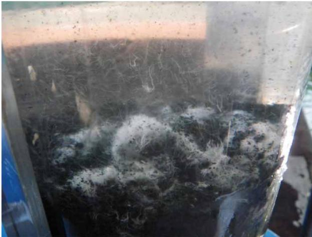
**Figure 4** | Photograph of the surface sediment sampled in Site 3 in July 2010. Inner diameter of the acrylic tube is 4 cm.
